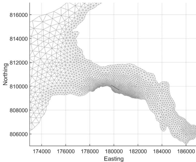
Figure 2. The unstructured mesh around the Loch Hourn site in the modified model grid, with the proposed cage locations indicated (•).
