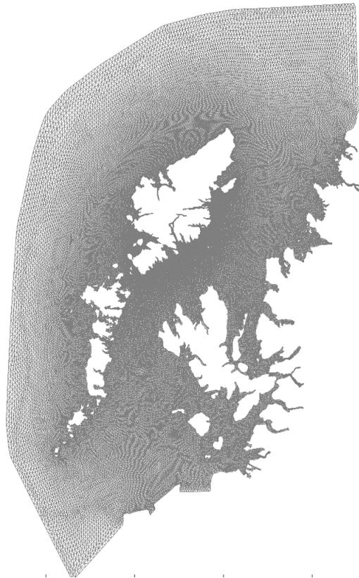
Figure 1. The mesh and domain of the East Coast of Lewis and Harris (ECLH) sub-model of the Scottish Shelf Model (Marine Scotland, 2016).
