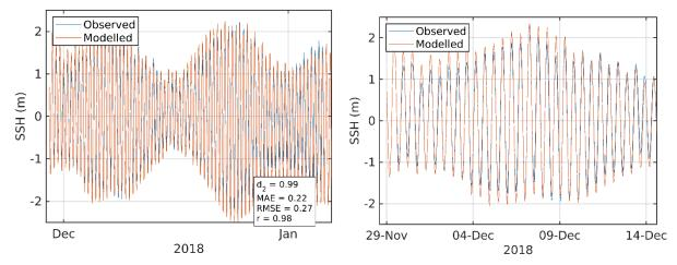
Figure 14. Comparison between observed and modelled sea surface height from November 2018 – February 2019 (ADCP deployment ID254) using model parameter values from Table 1. Both the full record (left) and a subset of 15 days (right) are shown. Observed data are in blue, model results in
