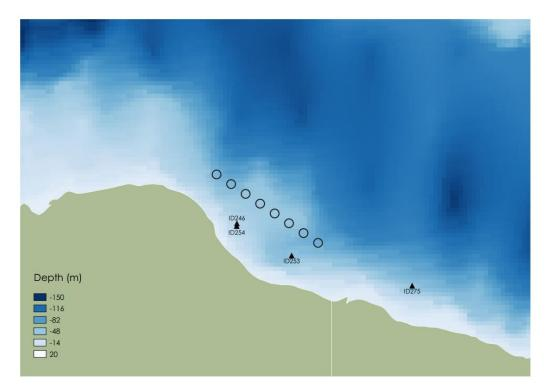
Figure 5. Locations of the ADCP deployments relative to the 8 pens at the Loch Hourn site.
