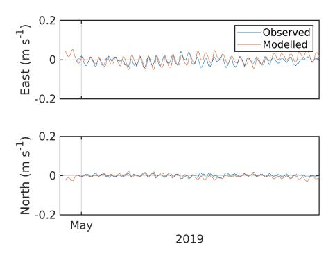
Figure 19. Comparison between observed and modelled East (top) and North (bottom) components of velocity at the ADCP location for 15 days in April – July 2019 (ID275). Observed data are in blue, model results in red.
