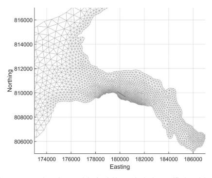
Figure 2. The unstructured mesh around the Loch Hourn site in the modified model grid, with the proposed cage locations indicated (•).
