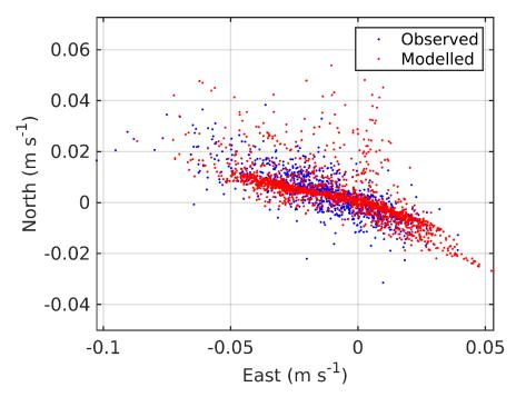
Figure 12. Scatter plot of observed and modelled velocity at the ADCP location from November 2018 – February 2019 (ID253). Observed data are in blue, model results in red.
