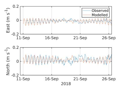
Figure 7. Comparison between observed and modelled East (top) and North (bottom) components of velocity at the ADCP location for 15 days in September – November 2018 (ID246). Observed data are in blue, model results in red.
