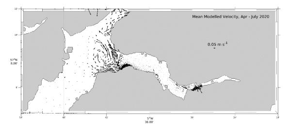
Figure 23. Mean modelled current vectors from 30<sup>th</sup> April – 4<sup>th</sup> July 2020 (ID275). For clarity, only 25% of the model vectors are shown, and vectors with a mean speed greater than 0.2 m s<sup>-1</sup> are also not shown
