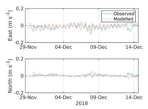
Figure 11. Comparison between observed and modelled East (top) and North (bottom) components of velocity at the ADCP location for 15 days in November 2018 – February 2019 (ID253). Observed data are in blue, model results in red.
