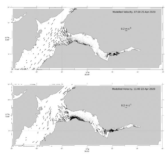
Figure 22. Modelled flood (top) and ebb (bottom) surface current vectors during spring tides on 25<sup>th</sup> April 2020 and 22<sup>nd</sup> April 2020 respectively. For clarity, only 25% of the model vectors are shown, and vectors with a speed greater than 0.3 m s<sup>-1</sup> are also not shown.
