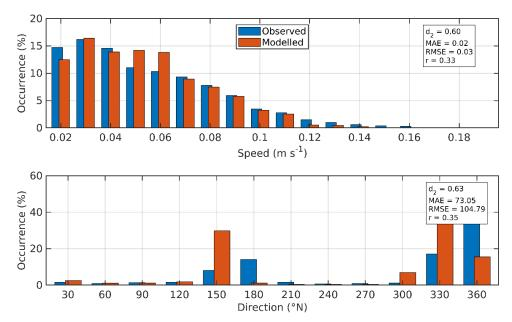
Figure 9. Histograms of observed and modelled speed (top) and direction (bottom) at the ADCP location from September – November 2018 (ID246). Observed data are in blue, model results in red.
