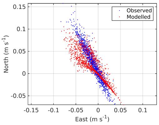
Figure 8. Scatter plot of observed and modelled velocity at the ADCP location from September – November 2018 (ID246). Observed data are in blue, model results in red.
