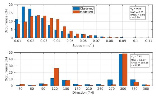
Figure 13. Histograms of observed and modelled current speed (top) and direction (bottom) at the ADCP location from November 2018 – February 2019 (ID253). Observed data are in blue, model results in red.
