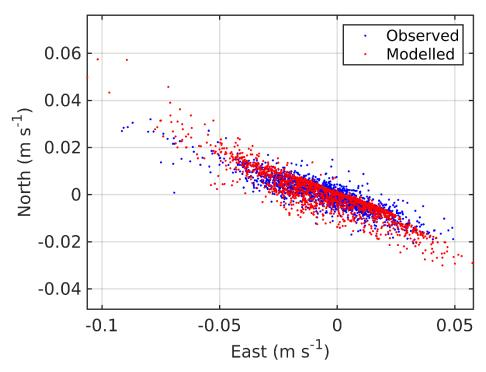
Figure 20. Scatter plot of observed and modelled velocity at the ADCP location from April – July 2019 (ID275). Observed data are in blue, model results in red.
