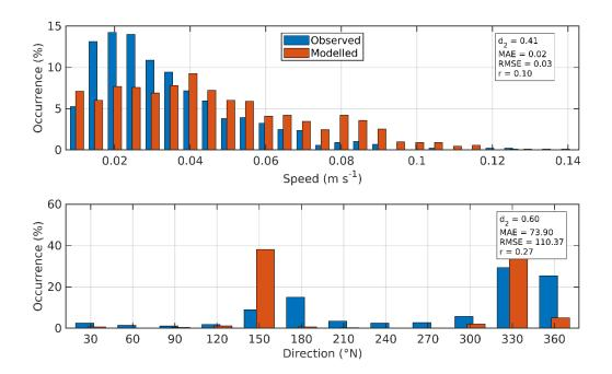
Figure 17. Histograms of observed and modelled current speed (top) and direction (bottom) at the ADCP location from November 2018 – February 2019 (ID254). Observed data are in blue, model results in red.
