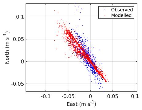
Figure 16. Scatter plot of observed and modelled velocity at the ADCP location from November 2018 – February 2019 (ID254). Observed data are in blue, model results in red.
