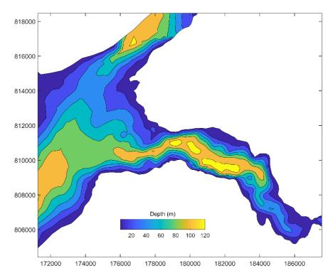
Figure 3. Model water depths (m) in the area around Loch Hourn salmon farm.
