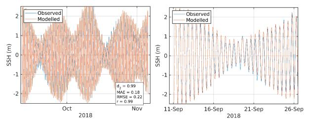
Figure 6. Comparison between observed and modelled sea surface height from September – November 2018 (ADCP deployment ID246) using model parameter values from Table 1Error!
