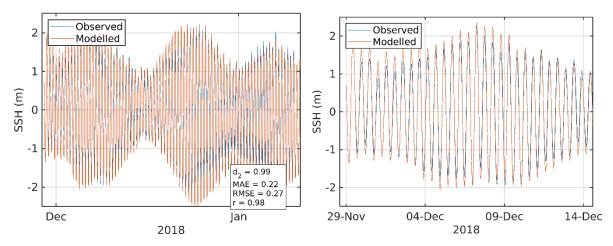
Figure 10. Comparison between observed and modelled sea surface height from November 2018 – February 2019 (ADCP deployment ID253) using model parameter values from Table 1. Both the full record (left) and a subset of 15 days (right) are shown. Observed data are in blue, model results in red.
