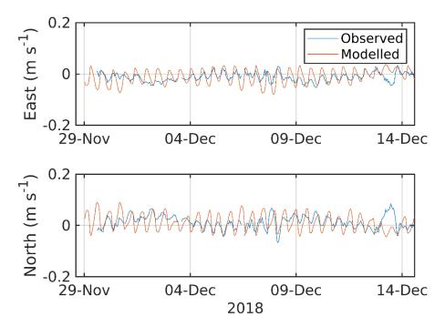
Figure 15. Comparison between observed and modelled East (top) and North (bottom) components of velocity at the ADCP location for 15 days in November 2018 – February 2019 (ID254). Observed data are in blue, model results in red.
