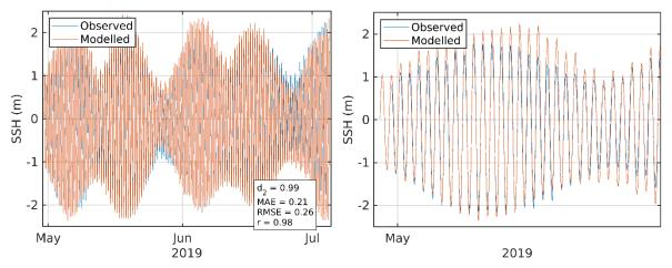
Figure 18. Comparison between observed and modelled sea surface height from April – July 2019 (ID275) using model parameter values from Table 1. Both the full record (left) and a subset of 15 days (right) are shown. Observed data are in blue, model results in red.
