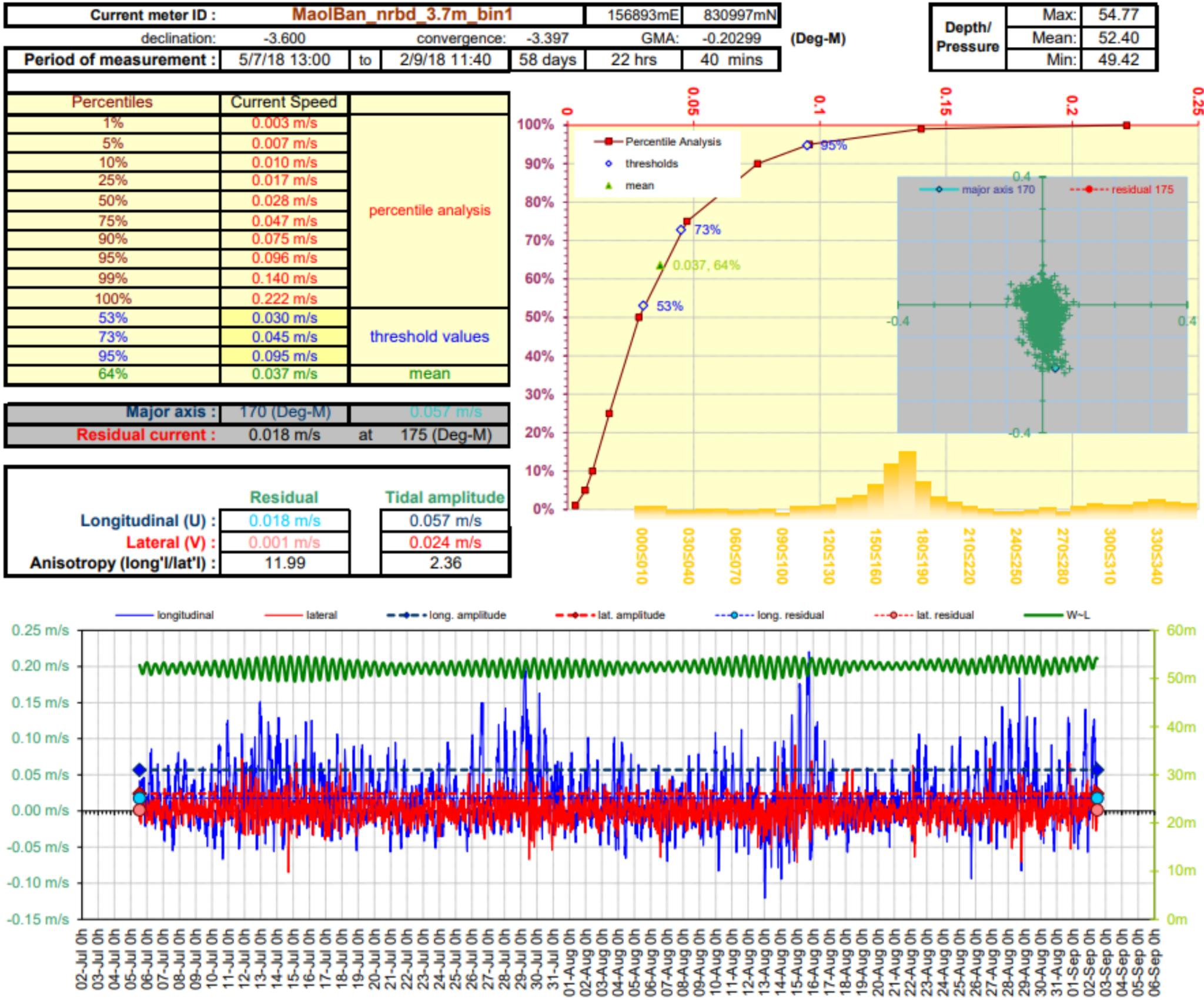
Figure 6. Current Data Summary Sheet for the near bottom current cell 1, 3.7m from seabed, 5<sup>th</sup> July to 2<sup>nd</sup> September 2018 inclusive (ID230).
