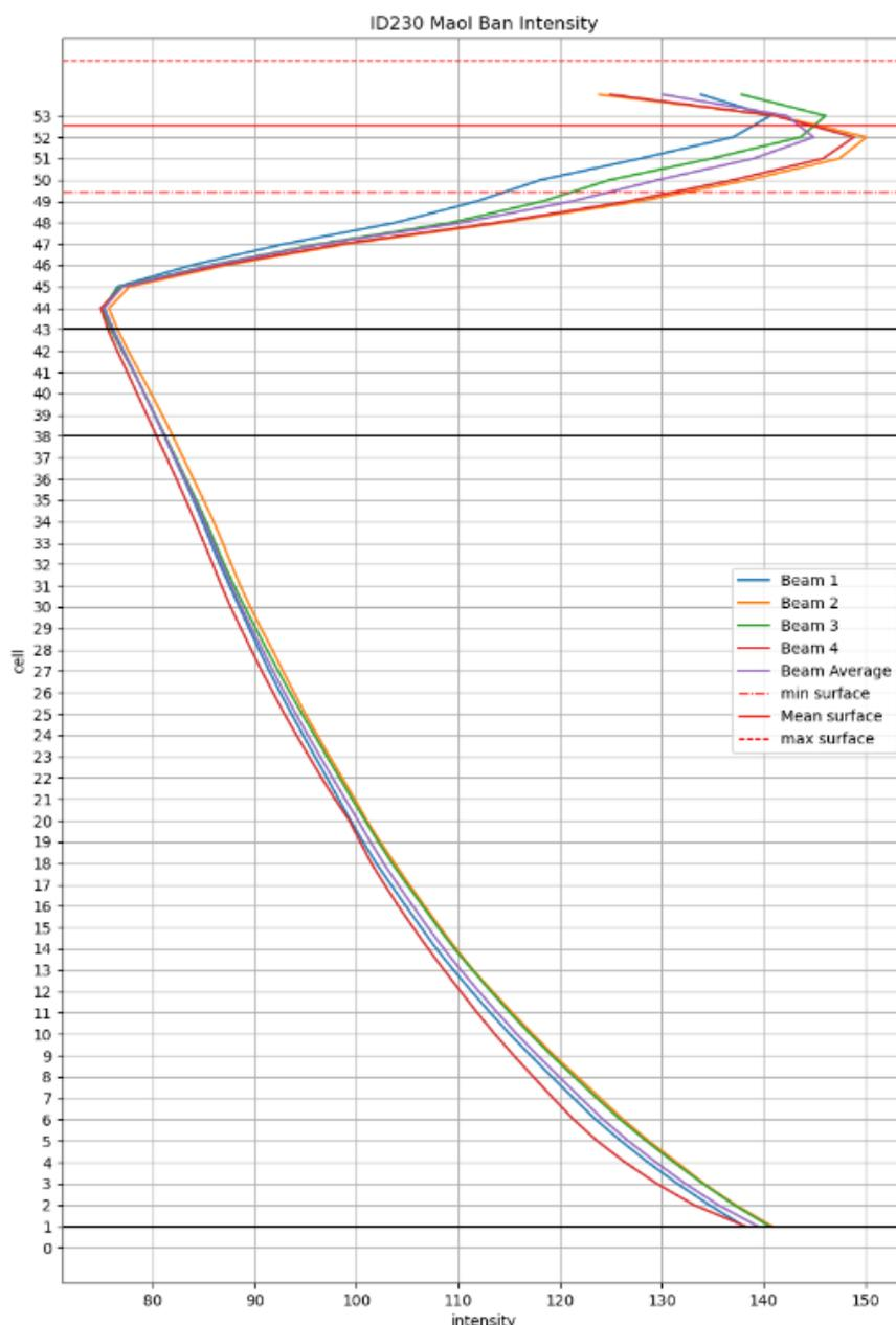
Figure 3. Mean intensity of the ADCP signal for the ID230 dataset plotted by bin number
