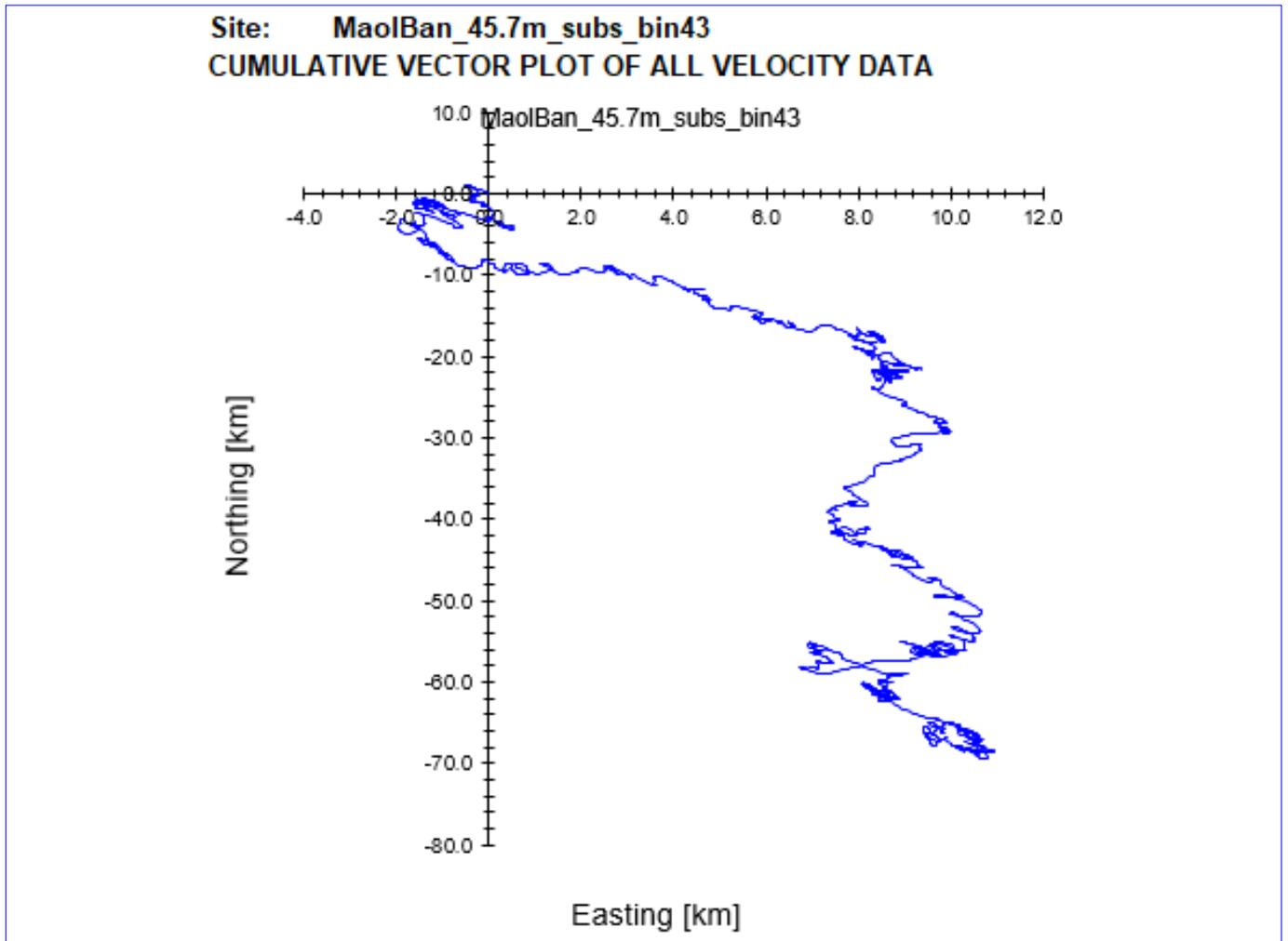
Figure 7. Cumulative Vector Plot of all velocity data from near surface cell for ID230.
