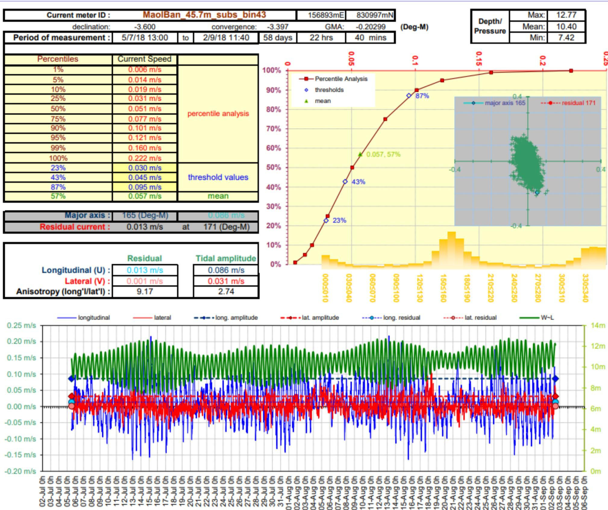
Figure 4. Current Data Summary Sheet for the surface current cell 43, 45.7m from seabed, 5<sup>th</sup> July to 2<sup>nd</sup> September 2018 inclusive (ID230).
