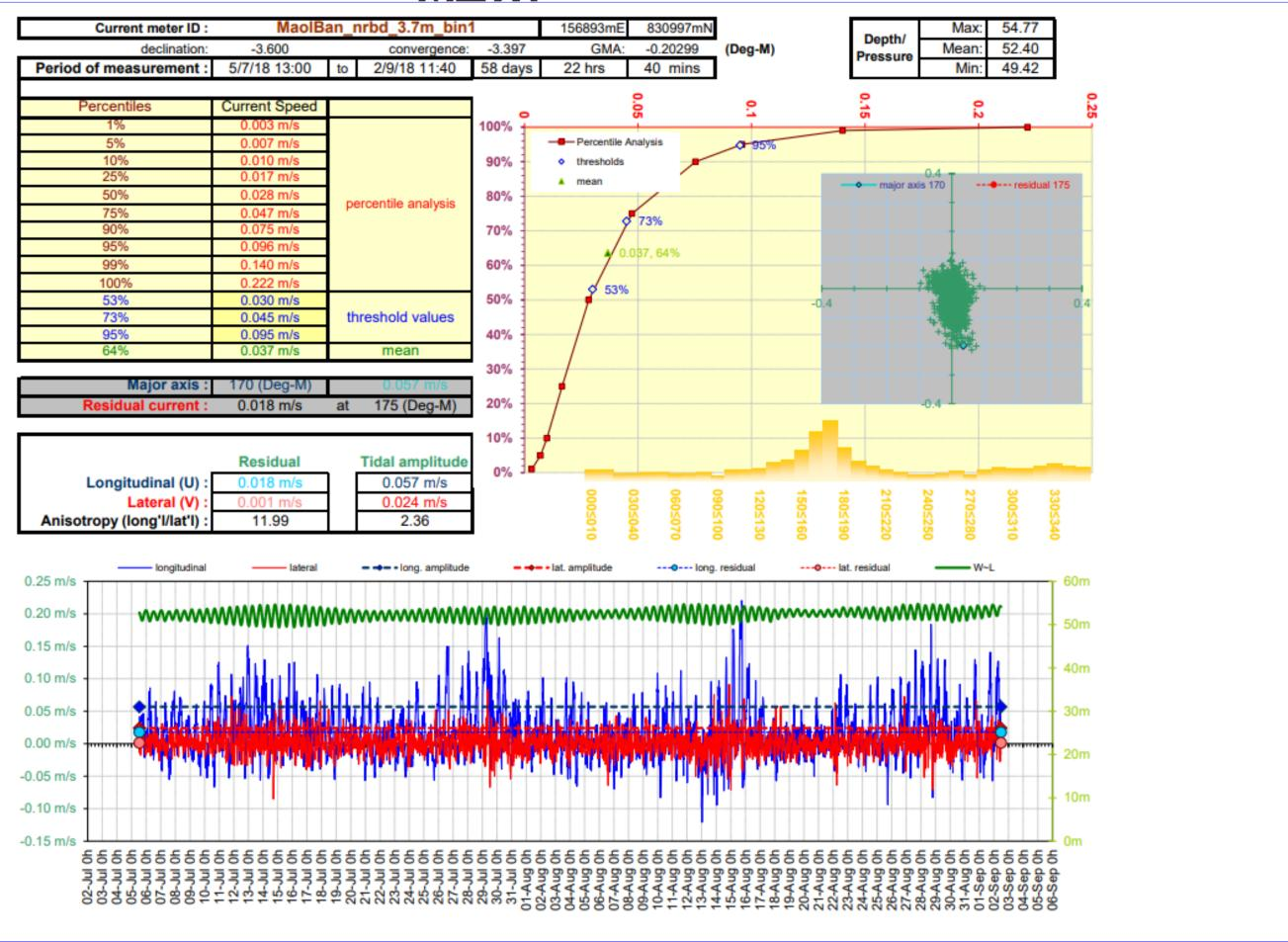
Figure 6. Current Data Summary Sheet for the near bottom current cell 1, 3.7m from seabed, 5th July to 2nd September 2018 inclusive (ID230).
