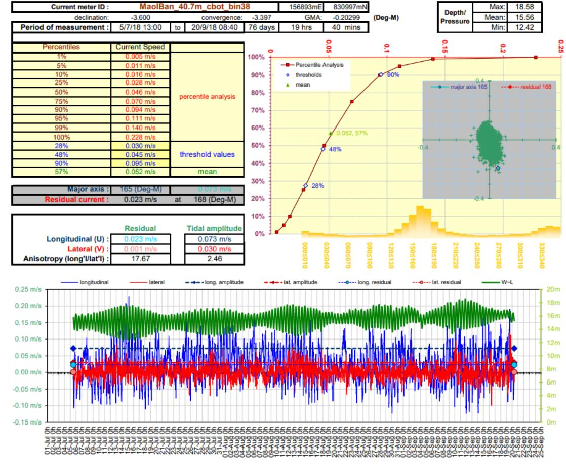
Figure 5. Current Data Summary Sheet for the cage bottom current cell 38, 40.7m from seabed, 5<sup>th</sup> July to 2<sup>nd</sup> September 2018 inclusive (ID230).
