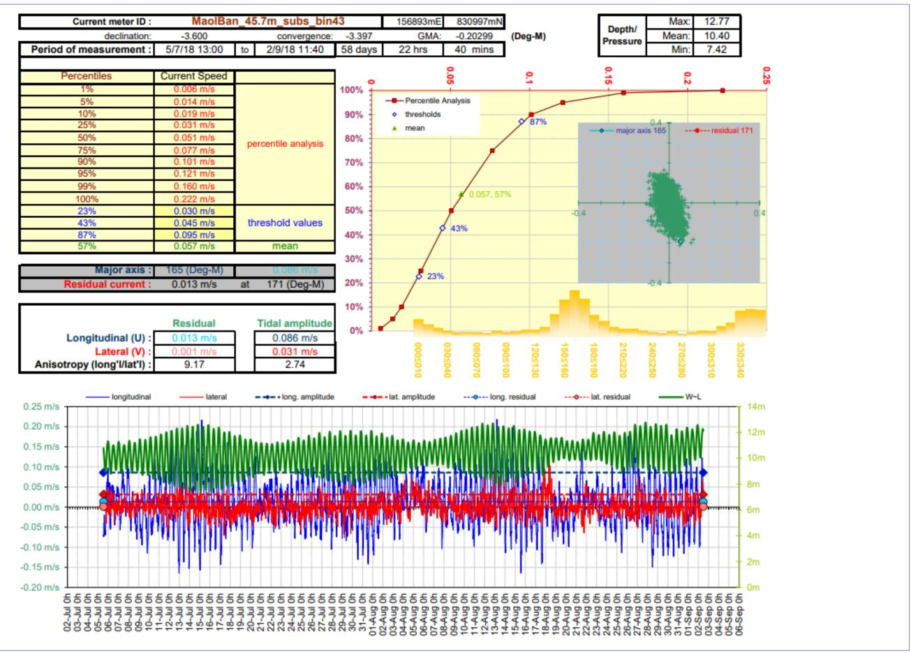
Figure 4. Current Data Summary Sheet for the surface current cell 43, 45.7m from seabed, 5th July to 2nd September 2018 inclusive (ID230).
