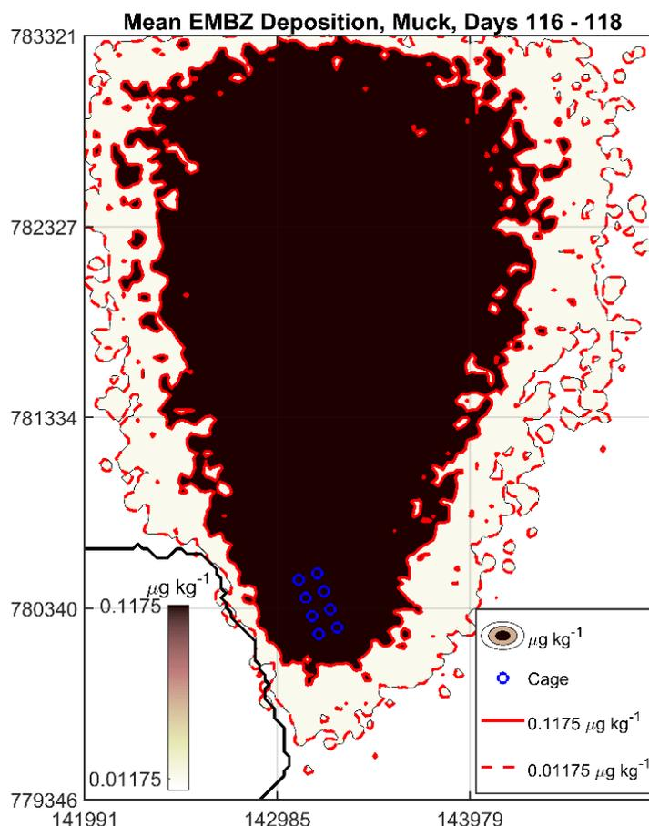
Figure 10: Predicted mean Emamectin Benzoate deposition over days 116-118 for the proposed 8 x 160m pens at Muck following a consented treatment of 1110g.
