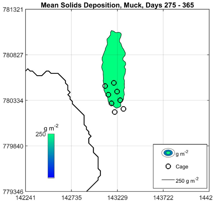
Figure 8. The modelled footprint for Muck for the proposed biomass increase of 4069 tonnes, using the SEPA standard default method.
