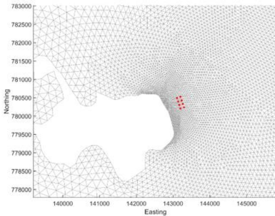
Figure 5. The unstructured mesh around the Muck site in the modified model grid, with the proposed pen locations indicated ( $\circ$ )
