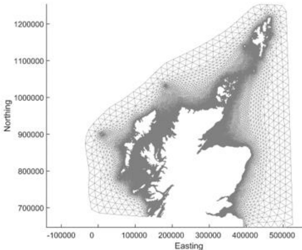
Figure 4. The mesh and domain of the modelling study, adapted from Gillibrand et al (2016b).
