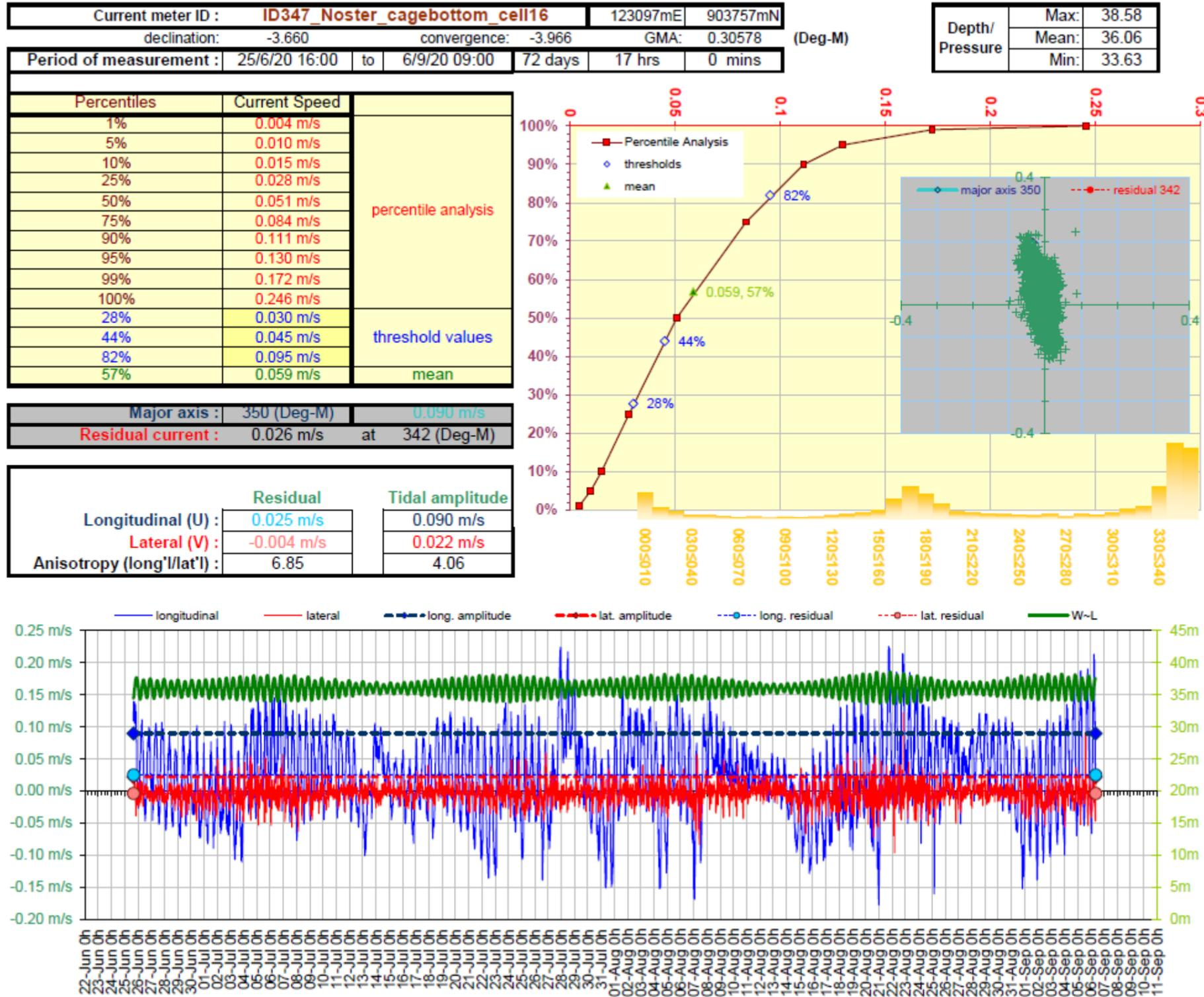
Figure 5. Current Data Summary Sheet for the cage bottom current cell 16, 34.68 m from seabed, 25<sup>th</sup> June to 6<sup>th</sup> September 2020 inclusive (ID347).
