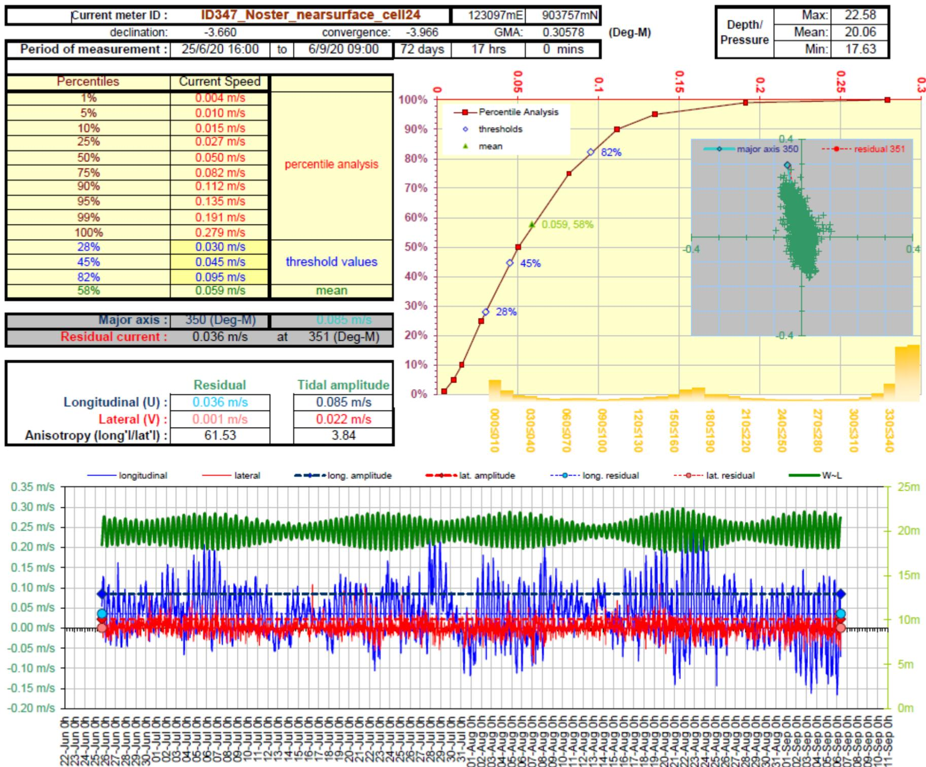
Figure 4. Current Data Summary Sheet for the surface current cell 24, 50.68 m from seabed, 25<sup>th</sup> June to 6<sup>th</sup> September 2020 inclusive (ID347).
