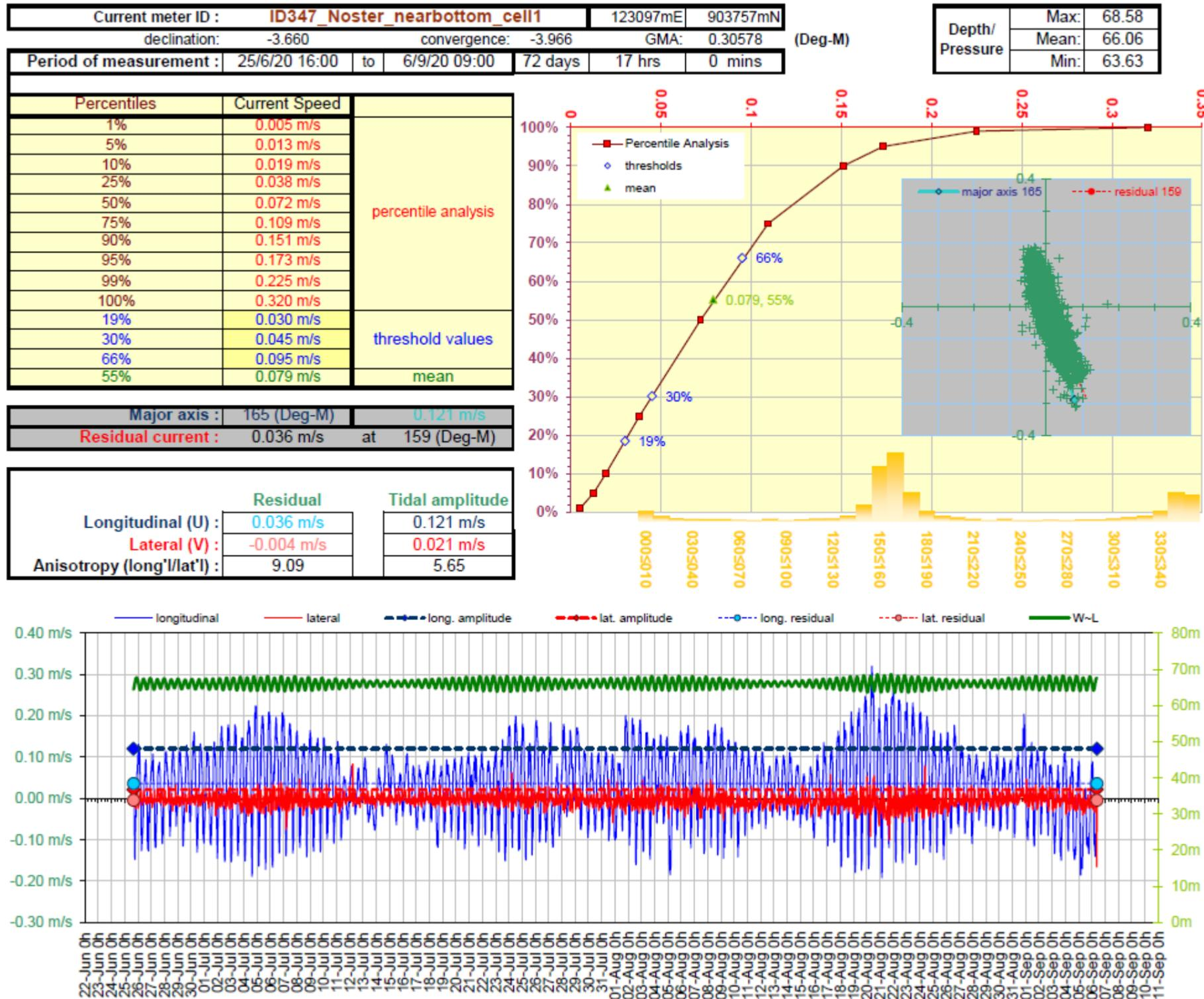
Figure 6. Current Data Summary Sheet for the near bottom current cell 1, 4.68m from seabed, 25<sup>th</sup> June to 6<sup>th</sup> September 2020 inclusive (ID347).
