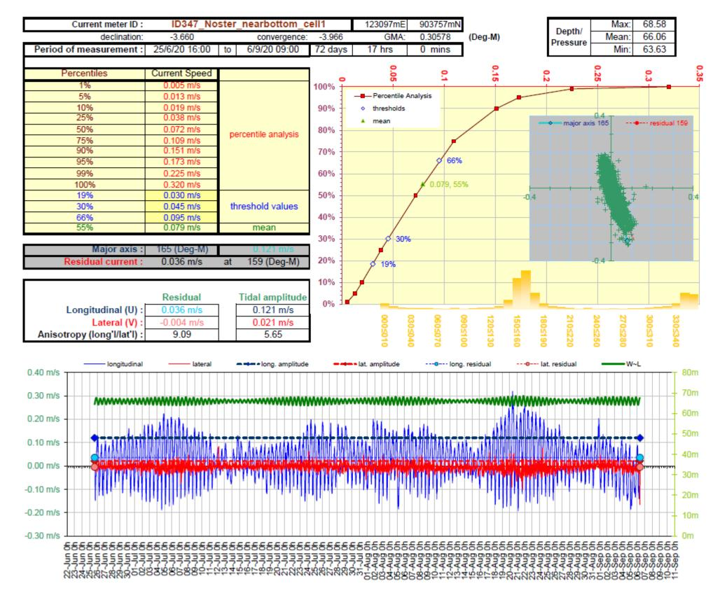
Figure 6. Current Data Summary Sheet for the near bottom current cell 1, 4.68m from seabed, 25th June to 6th September 2020 inclusive (ID347).
