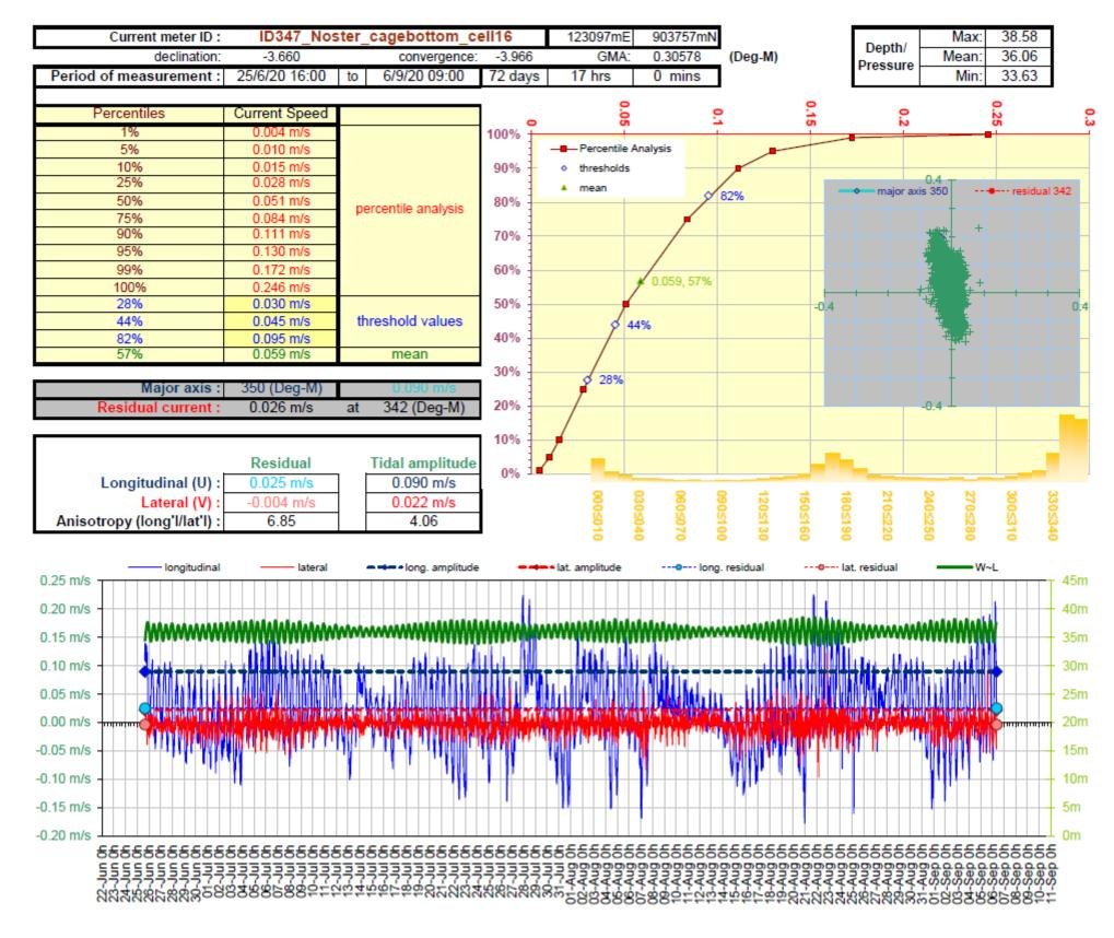
Figure 5. Current Data Summary Sheet for the cage bottom current cell 16, 34.68 m from seabed, 25th June to 6th September 2020 inclusive (ID347).
