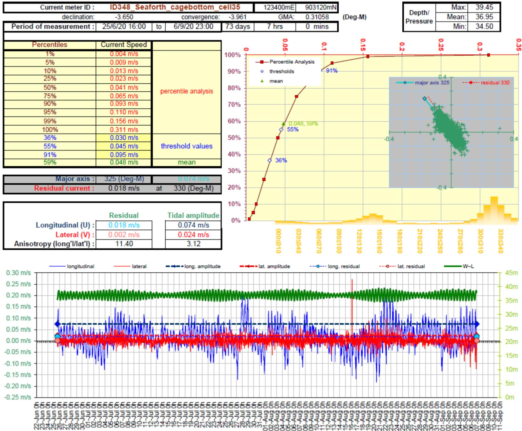
Figure 5. Current Data Summary Sheet for the cage bottom current cell 35, 72.68 m from seabed, 25<sup>th</sup> June to 6<sup>th</sup> September 2020 inclusive (ID348).
