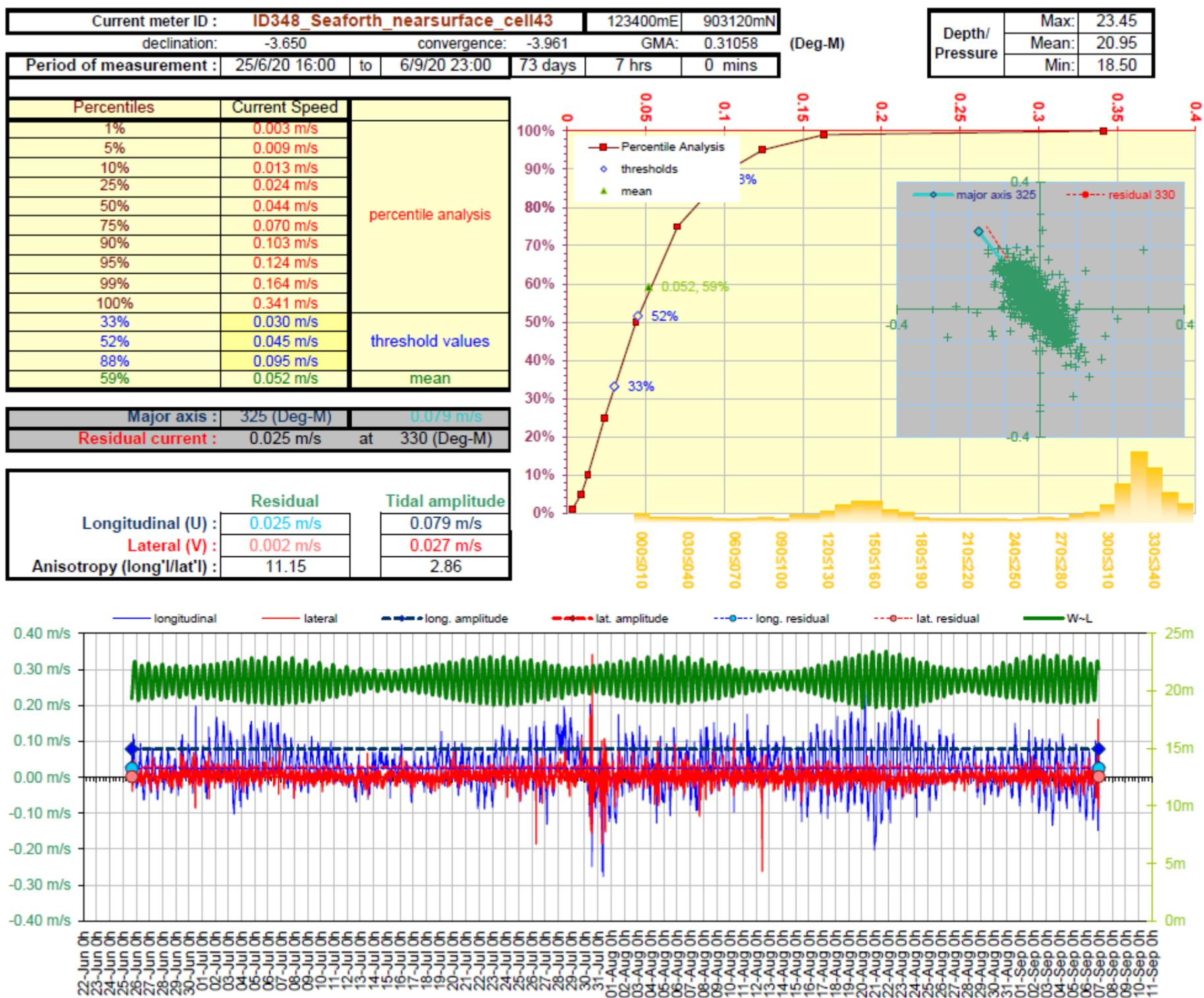
Figure 4. Current Data Summary Sheet for the surface current cell 43, 88.68 m from seabed, 25<sup>th</sup> June to 6<sup>th</sup> September 2020 inclusive (ID348).
