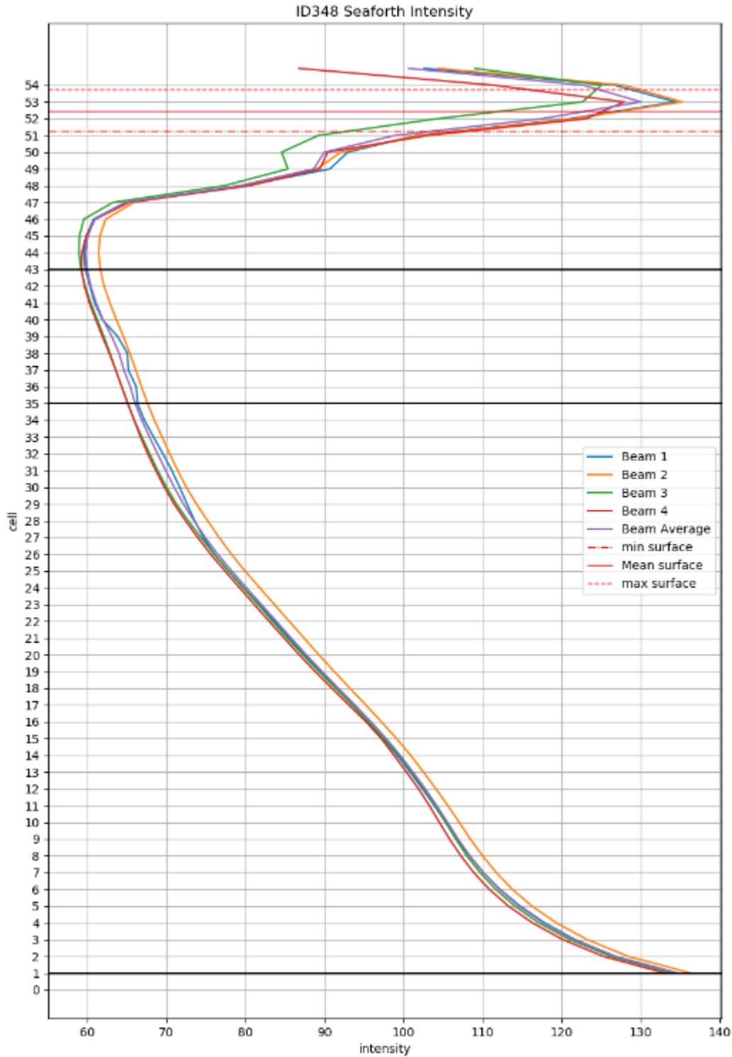
Figure 3. Mean intensity of the ADCP signal for the ID328 dataset plotted by bin number
