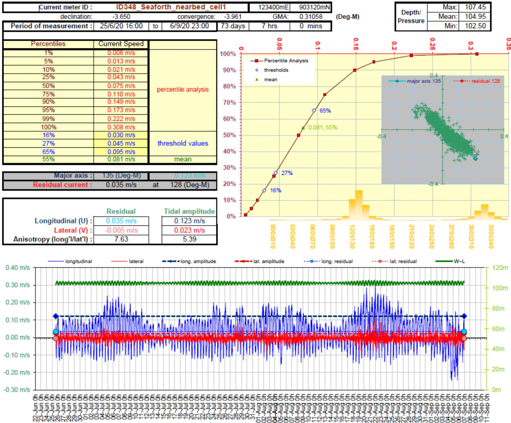
Figure 6. Current Data Summary Sheet for the near bottom current cell 1, 4.68m from seabed, 25<sup>th</sup> June to 6<sup>th</sup> September 2020 inclusive (ID348).
