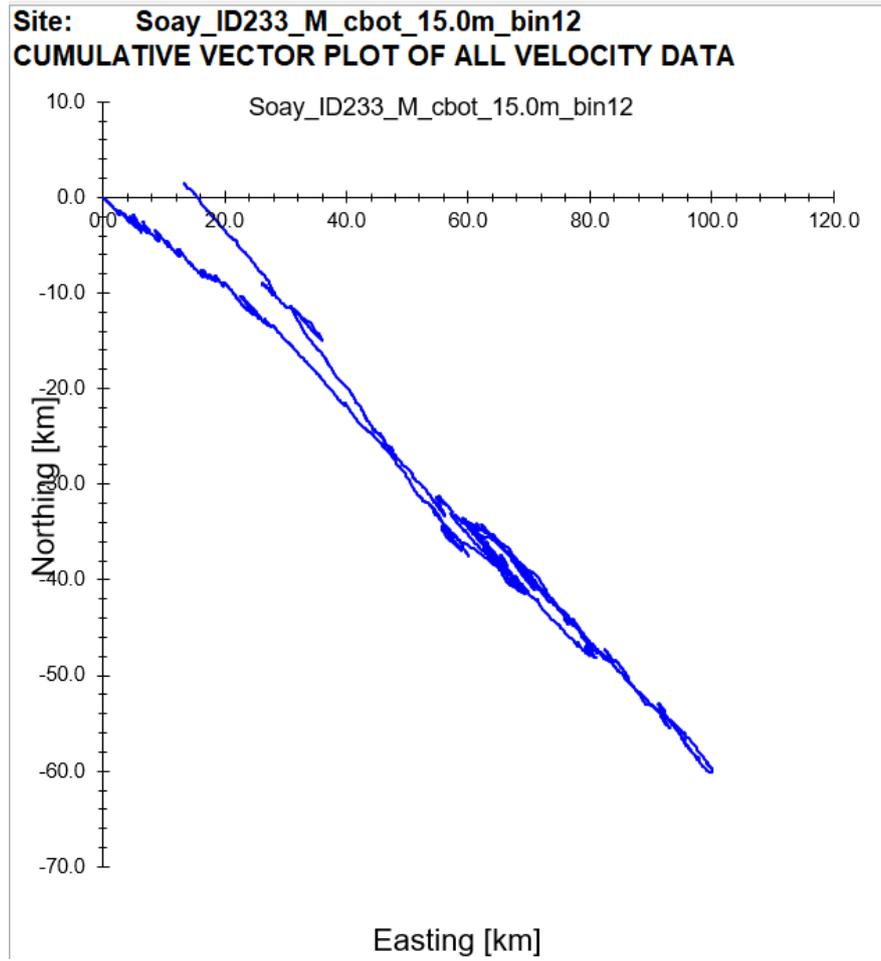
Figure 10. Cumulative Vector Plot of all velocity data from cage bottom cell for ID233.
