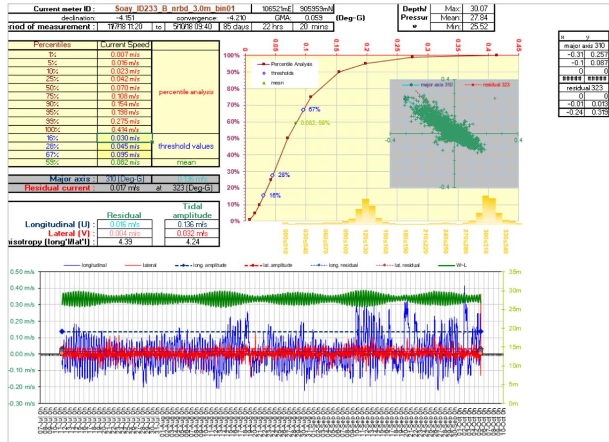
Figure 8. Current Data Summary Sheet for the near bottom current cell 01, 3.72m from seabed, 11<sup>th</sup> July to 18<sup>th</sup> October 2018 inclusive (ID233).
