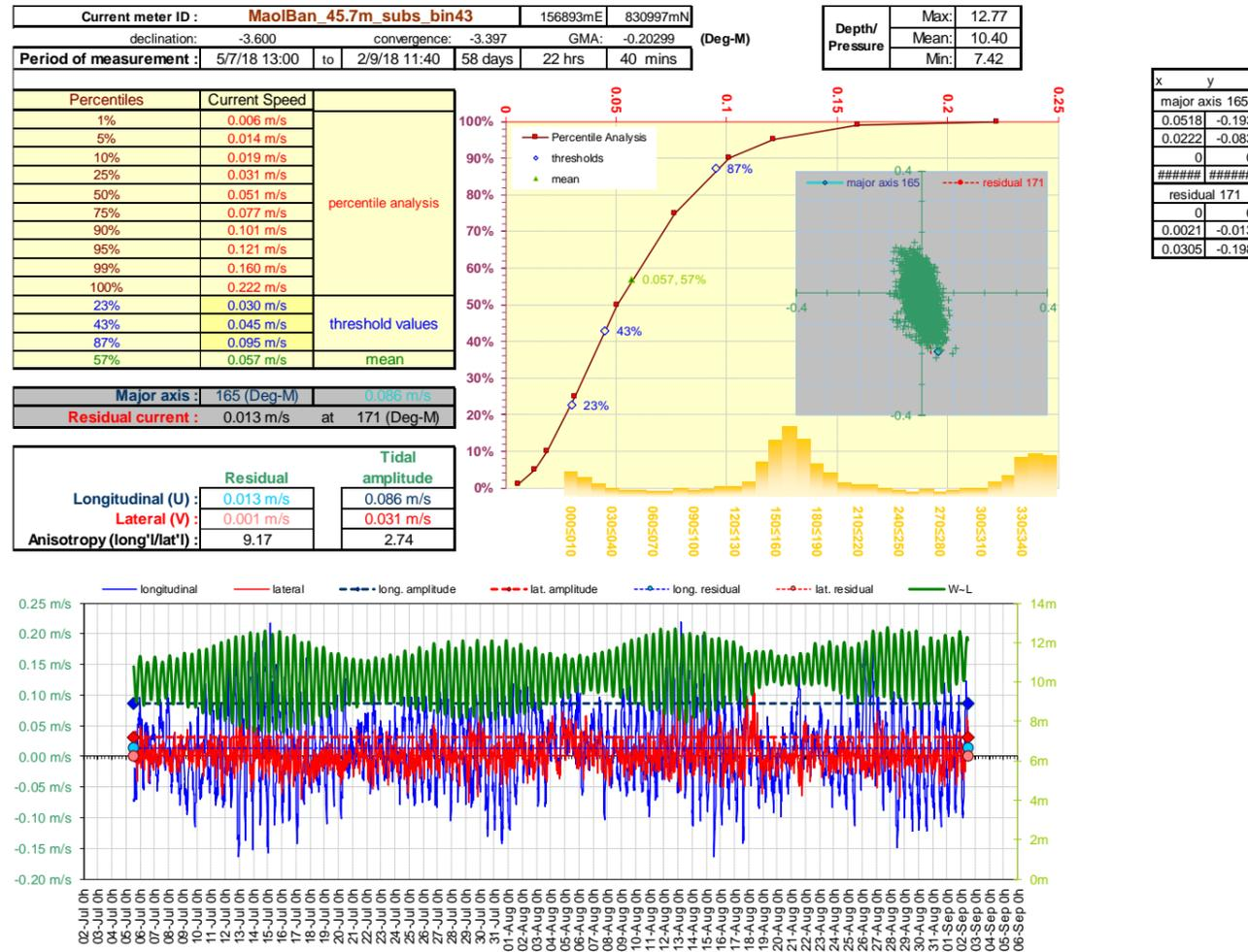
Figure 6. Current Data Summary Sheet for the surface current cell 26, 25.72m from seabed, 11<sup>th</sup> July to 18<sup>th</sup> October 2018 inclusive (ID233).
