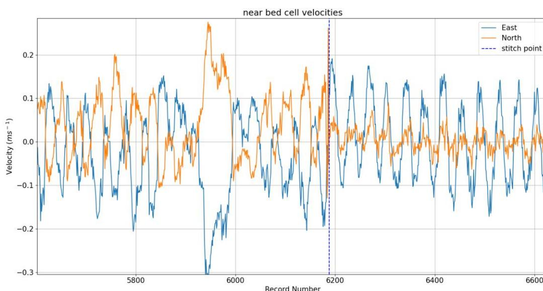
Figure 5. Near bed cell velocities East and North centered around the stitching point of the two current meter records
