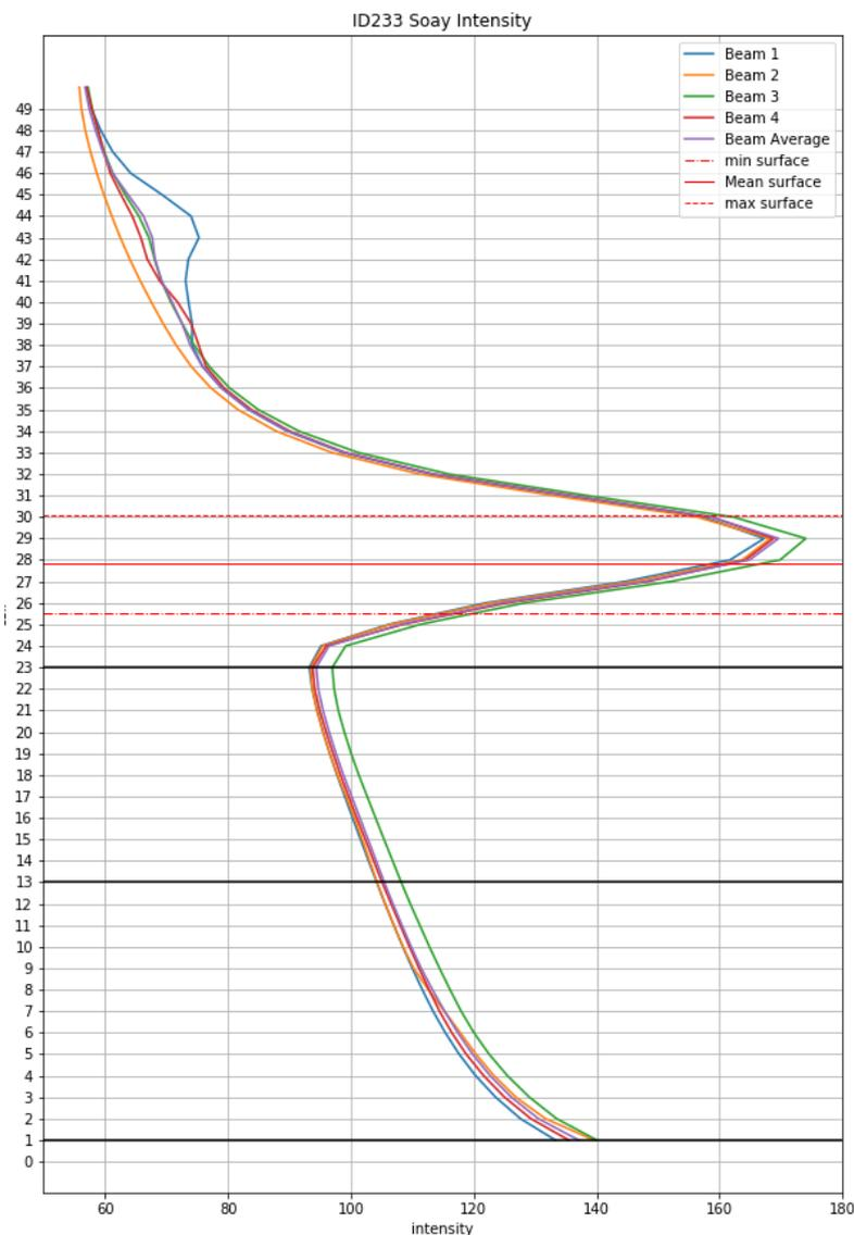
Figure 3. Mean intensity of the ADCP signal for the ID233 dataset plotted by cell
