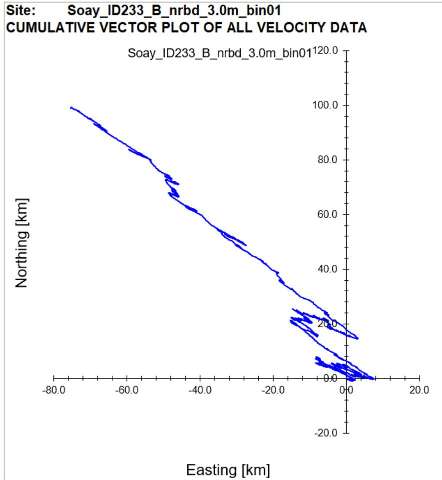
Figure 11. Cumulative Vector Plot of all velocity data from near bottom cell for ID233.
