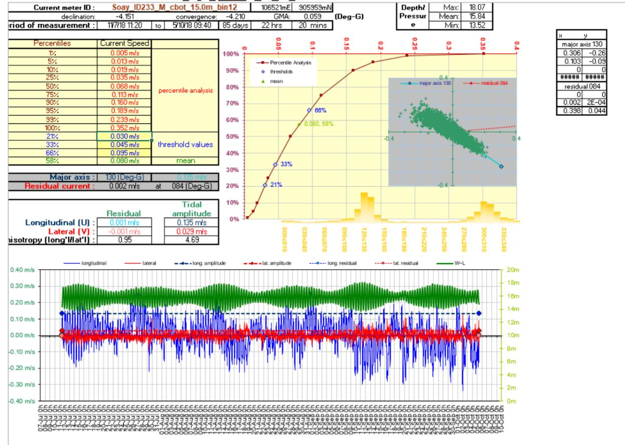
Figure 7. Current Data Summary Sheet for the cage bottom current cell 12, 15.72m from seabed, 11<sup>th</sup> July to 18<sup>th</sup> October 2018 inclusive (ID366).
