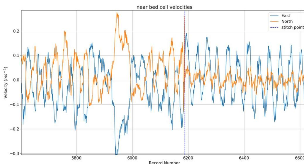
Figure 4. Near bed cell velocities East and North from complete flowmetry file with stitch point indicated with a blue dotted vertical line
