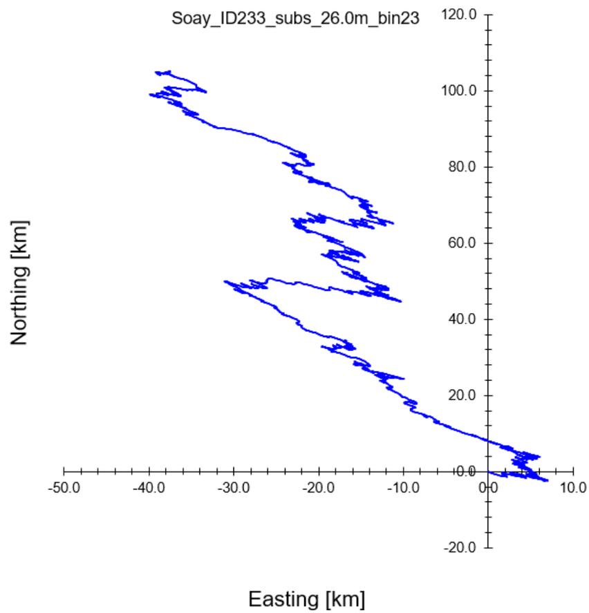
Figure 9. Cumulative Vector Plot of all velocity data from near surface cell for ID233.
