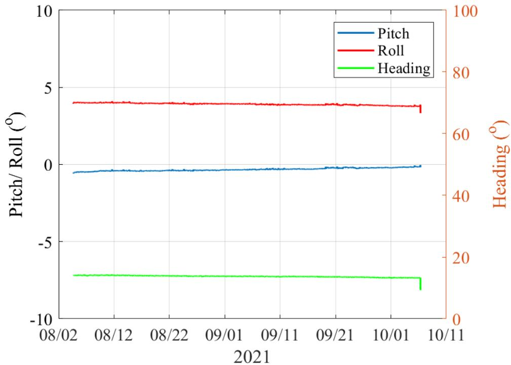
Figure 0.2. Pitch, roll and heading for North Gravir deployment 1, from 04/08/2021 - 06/10/2021.
