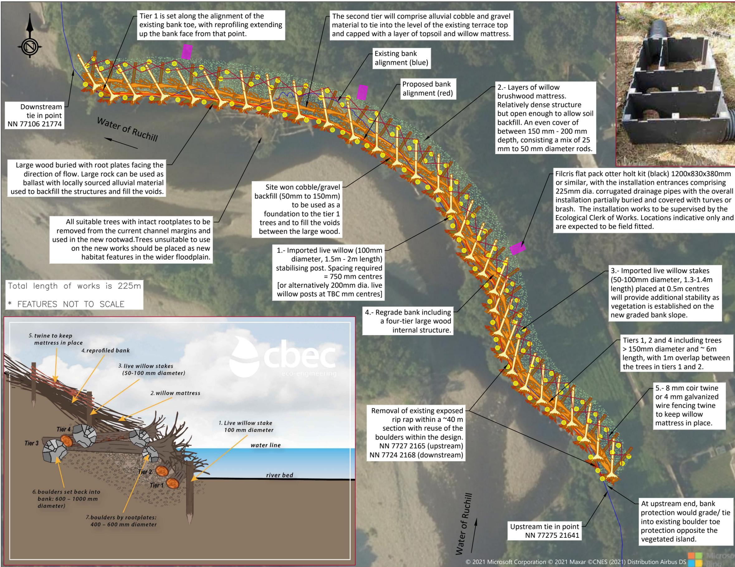
Large wood buried with root plates facing the direction of flow. Large rock can be used as ballast with locally sourced alluvial material used to backfill the structures and fill the voids.
