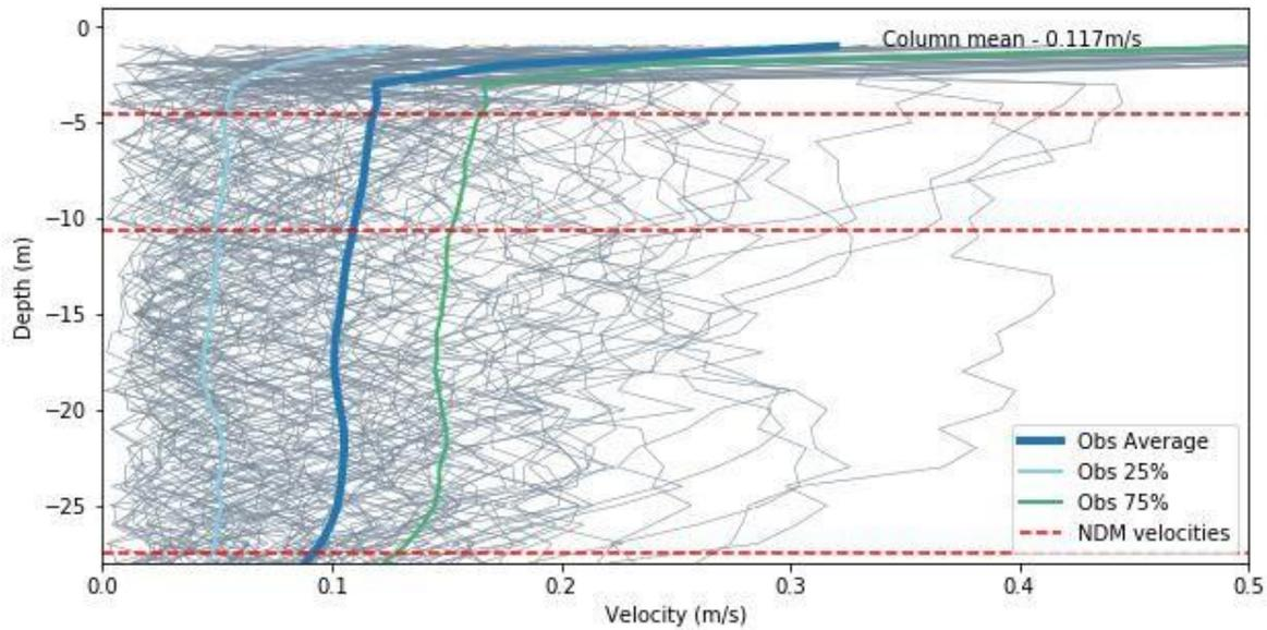
**Figure 3.1: Sampled velocity profiles for the hydrographic deployment used in this assessment**
