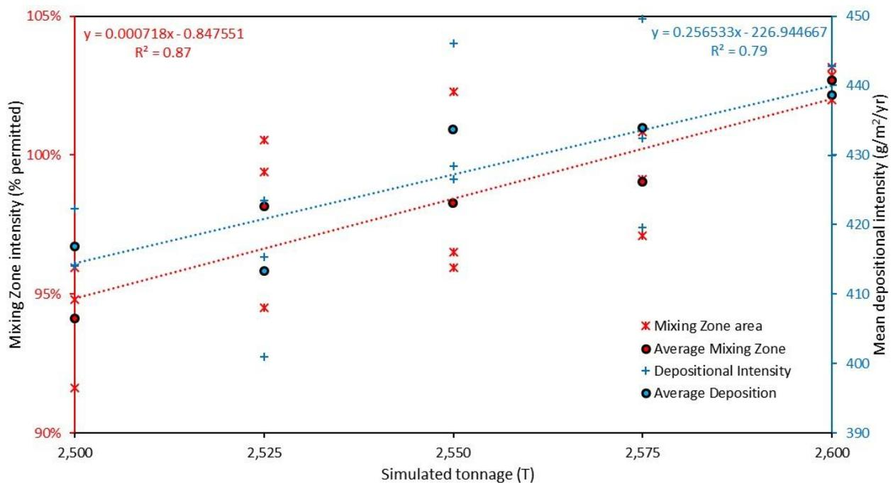
**Figure 4.1: De-trended, scoping runs used to define maximum permissible tonnage. NB: each tonnage was run in triplicate and an average taken (mitigating Fickian processes within the modelling framework)**
