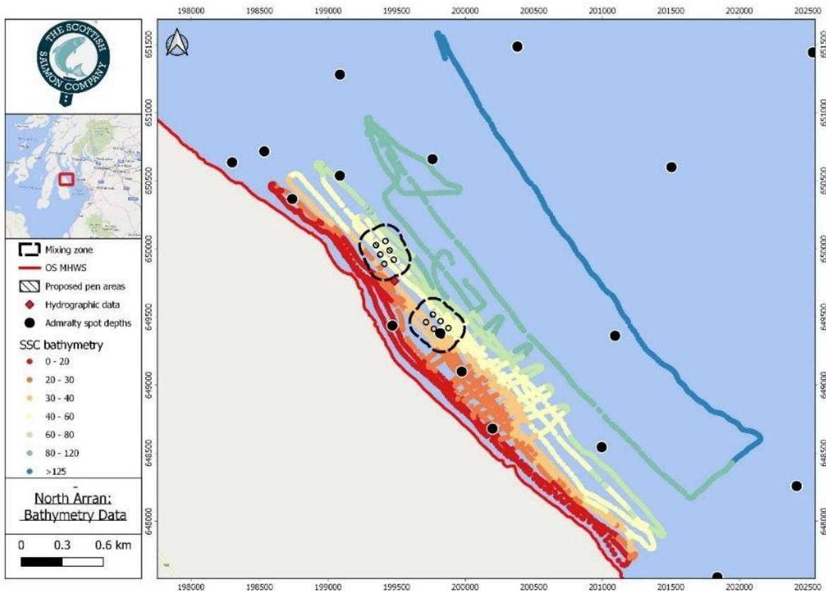
Figure 3.5: Bathymetry data available at the North Arran Site
