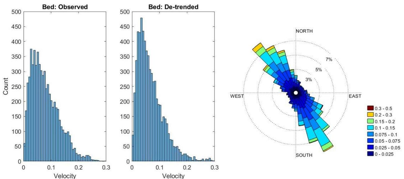
**Figure 3.4: Velocity distribution plots for the bed from observed and De-trended datasets (left) and the Detrended bed rose, derived from the 90-day observed dataset (right)**
