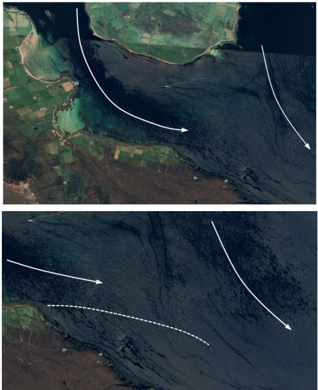
Figure 3.12 Satellite imagery showing the flood tide flows around Graemsay (top) and how they interact close to the Bring Head site (bottom)
