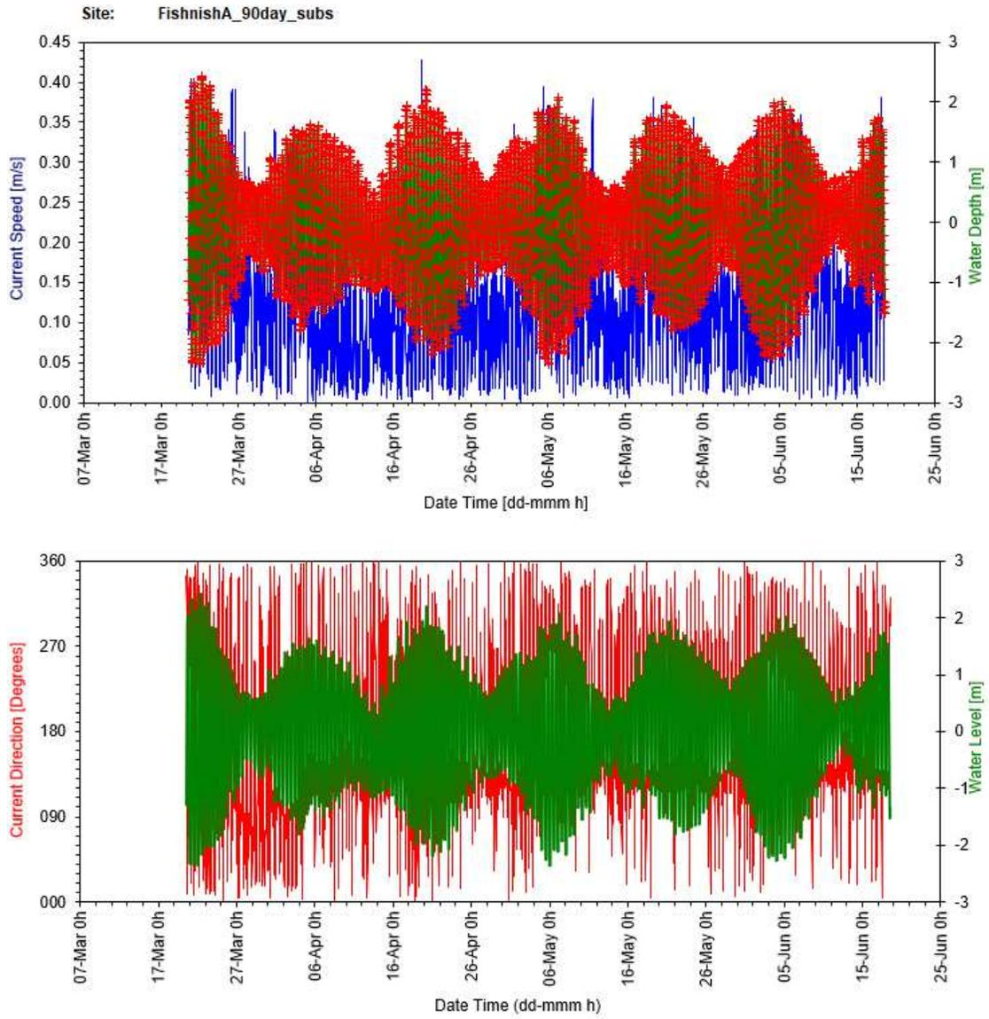
Figure 34: Subsurface time series plots for current speed and direction against water level
