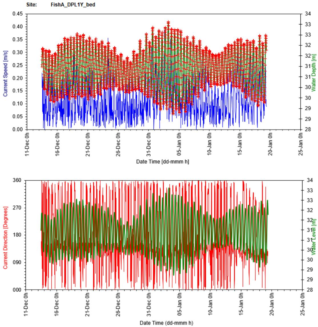
Figure 14: Near-bed time series plots for current speed and direction against water level
