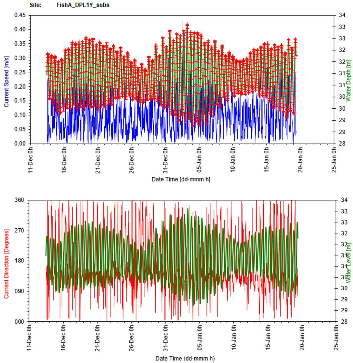
Figure 16: Subsurface time series plots for current speed and direction against water level
