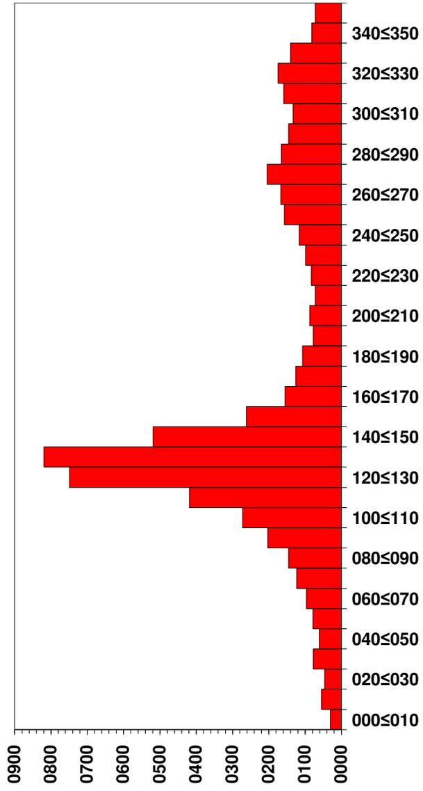
Figure 40: Subsurface current direction frequency plot.
