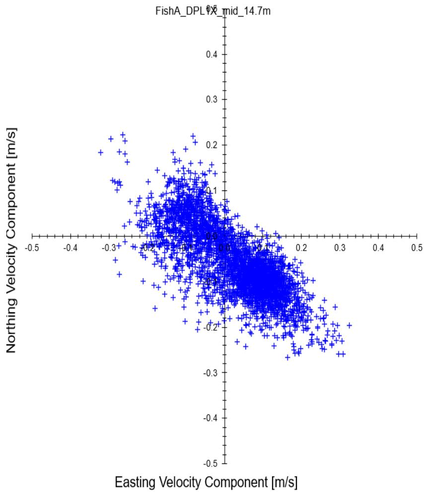
Figure 27: Cage bottom scatter plot of easting and northing velocity components
