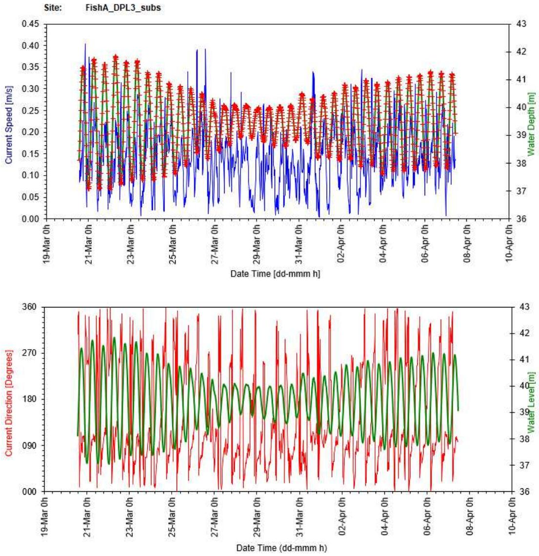
Figure 7: Subsurface time series plots for current speed and direction against water level
