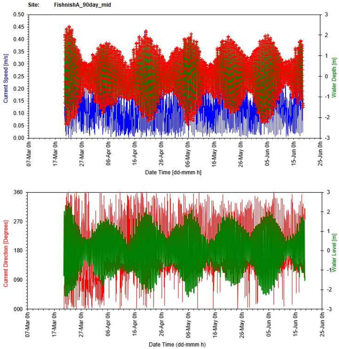
Figure 33: Mid time series plots for current speed and direction against water level
