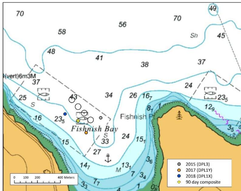
Figure 3: Recorded location of Fishnish 2015, 2017 & 2018 current meter deployments and the 90 day composite position used for NewDepomod modelling
