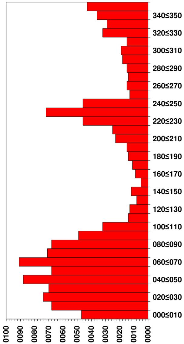
Figure 11: Near-bed current direction frequency plot.
