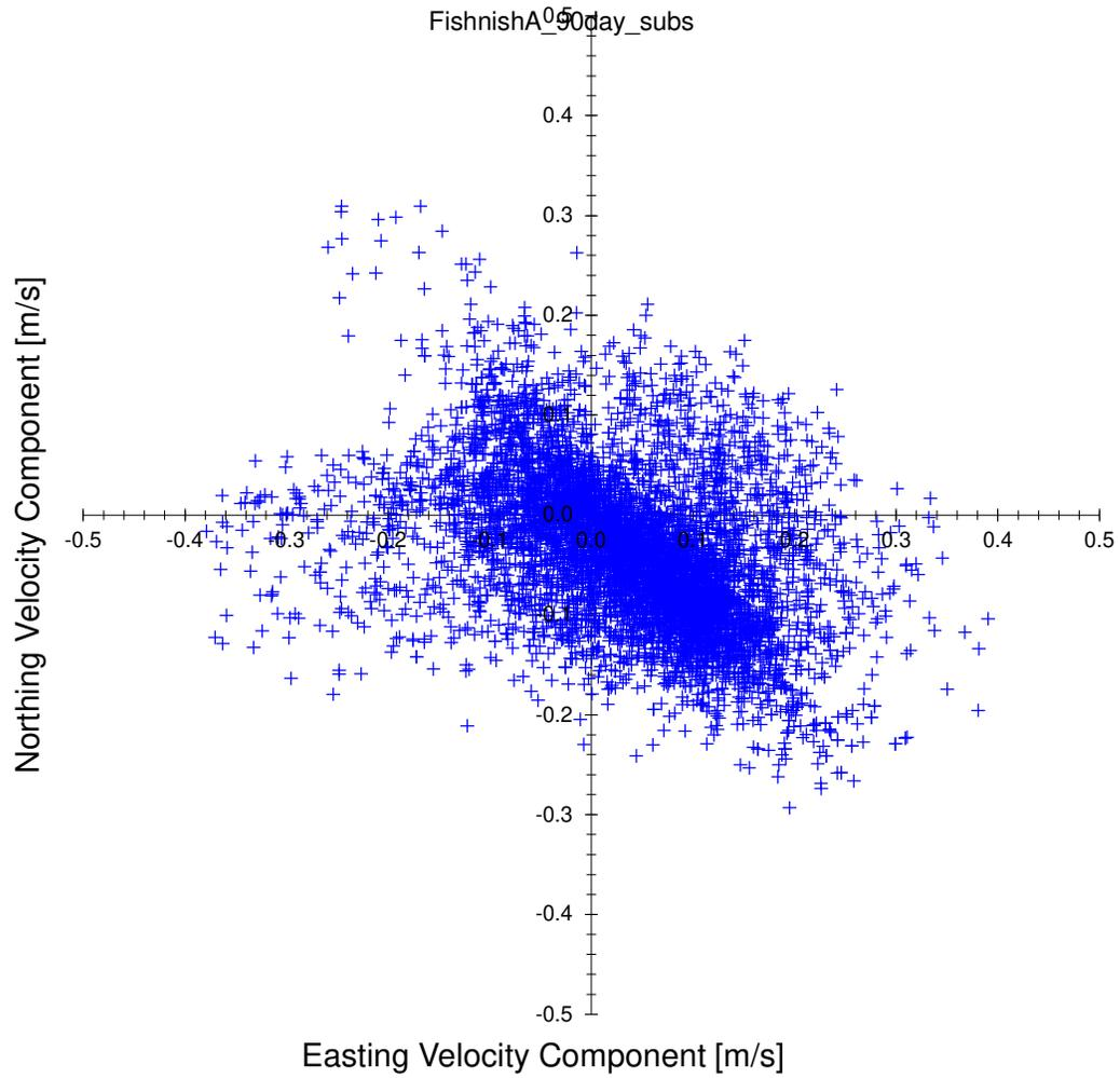
Figure 37: Subsurface scatter plot of easting and northing velocity components
