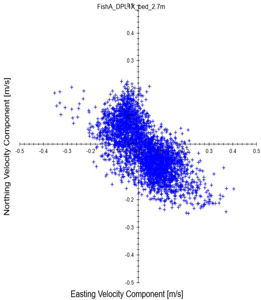
Figure 26: Near-bed scatter plot of easting and northing velocity components
