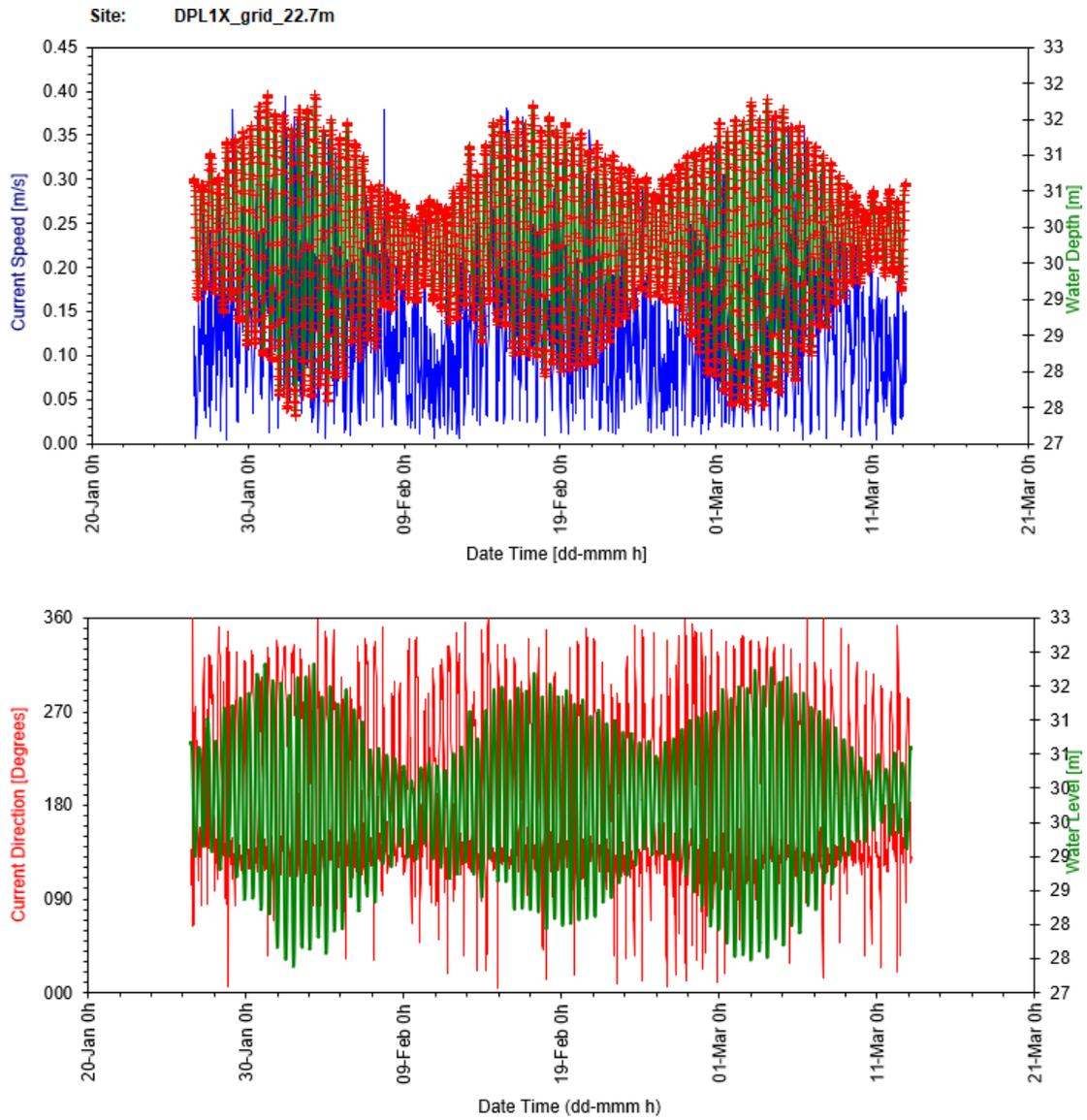
Figure 25: Subsurface time series plots for current speed and direction against water level
