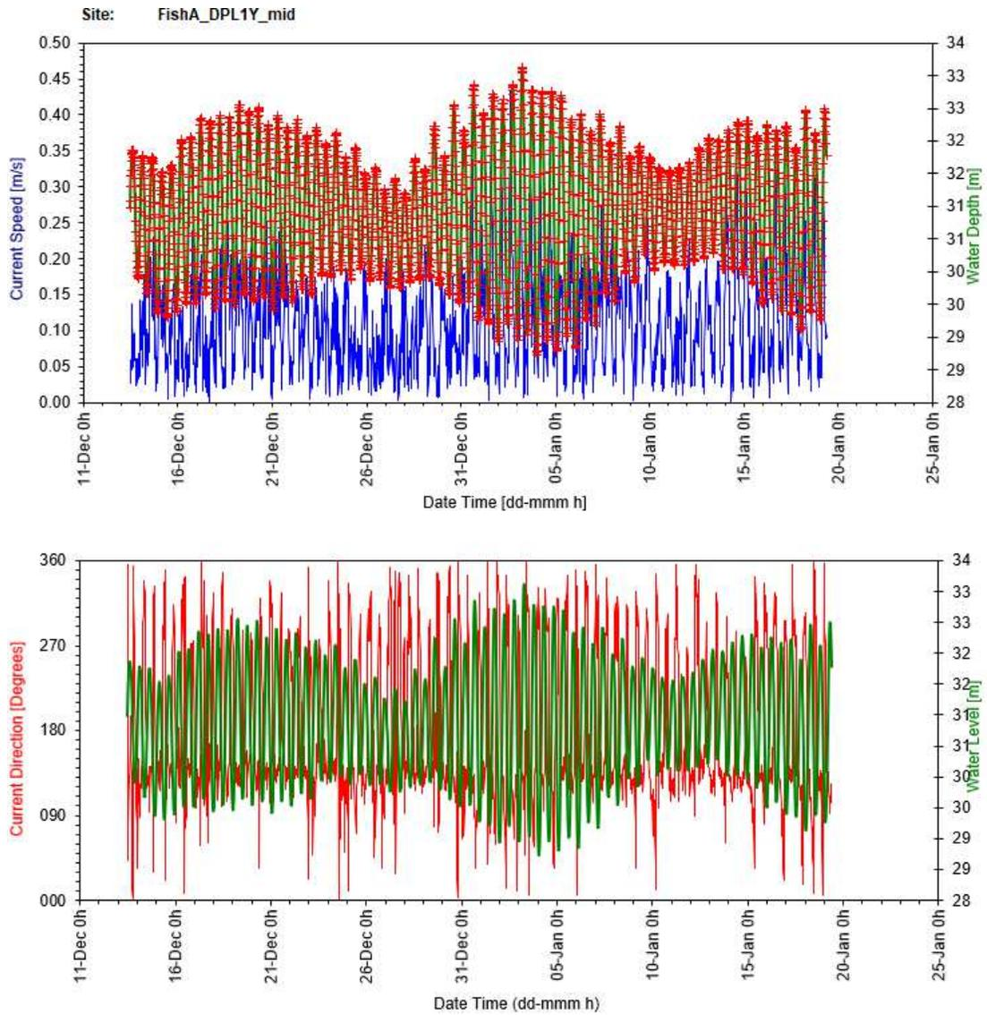
Figure 15: Cage bottom time series plots for current speed and direction against water level
