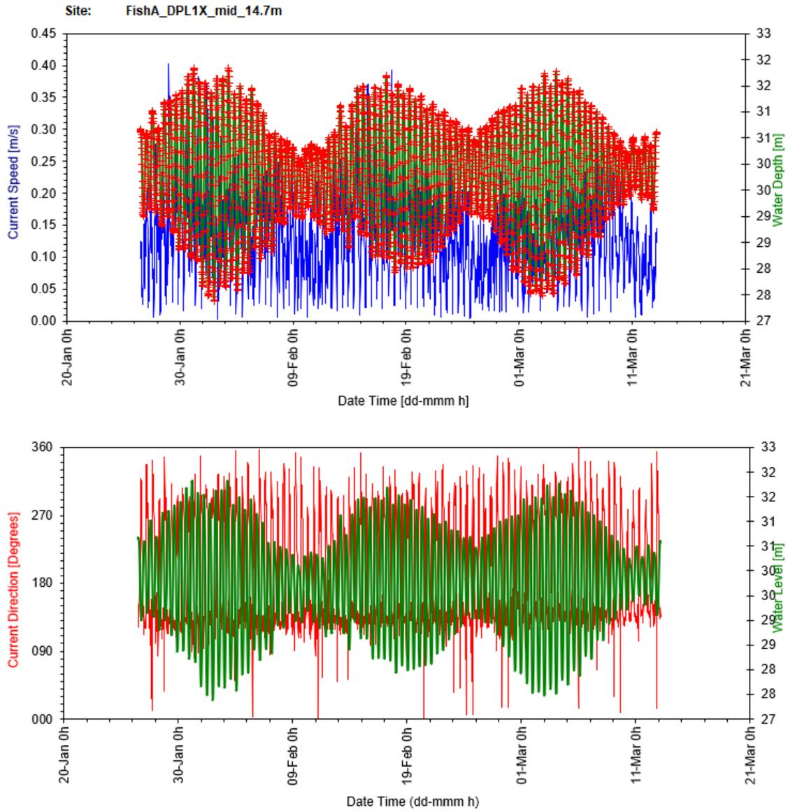
Figure 24: Cage bottom time series plots for current speed and direction against water level
