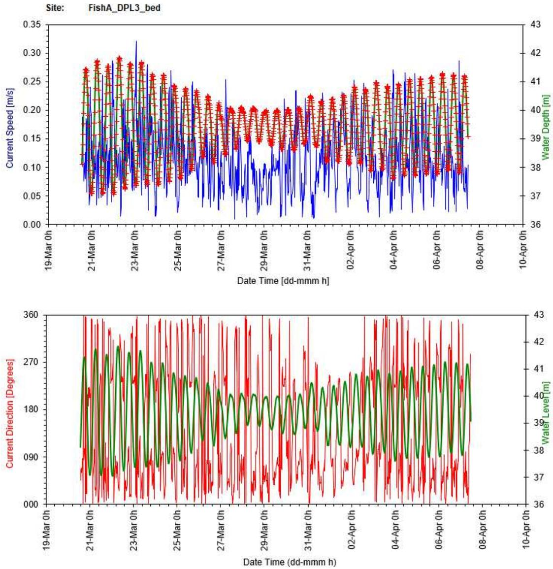
Figure 5: Near-bed time series plots for current speed and direction against water level
