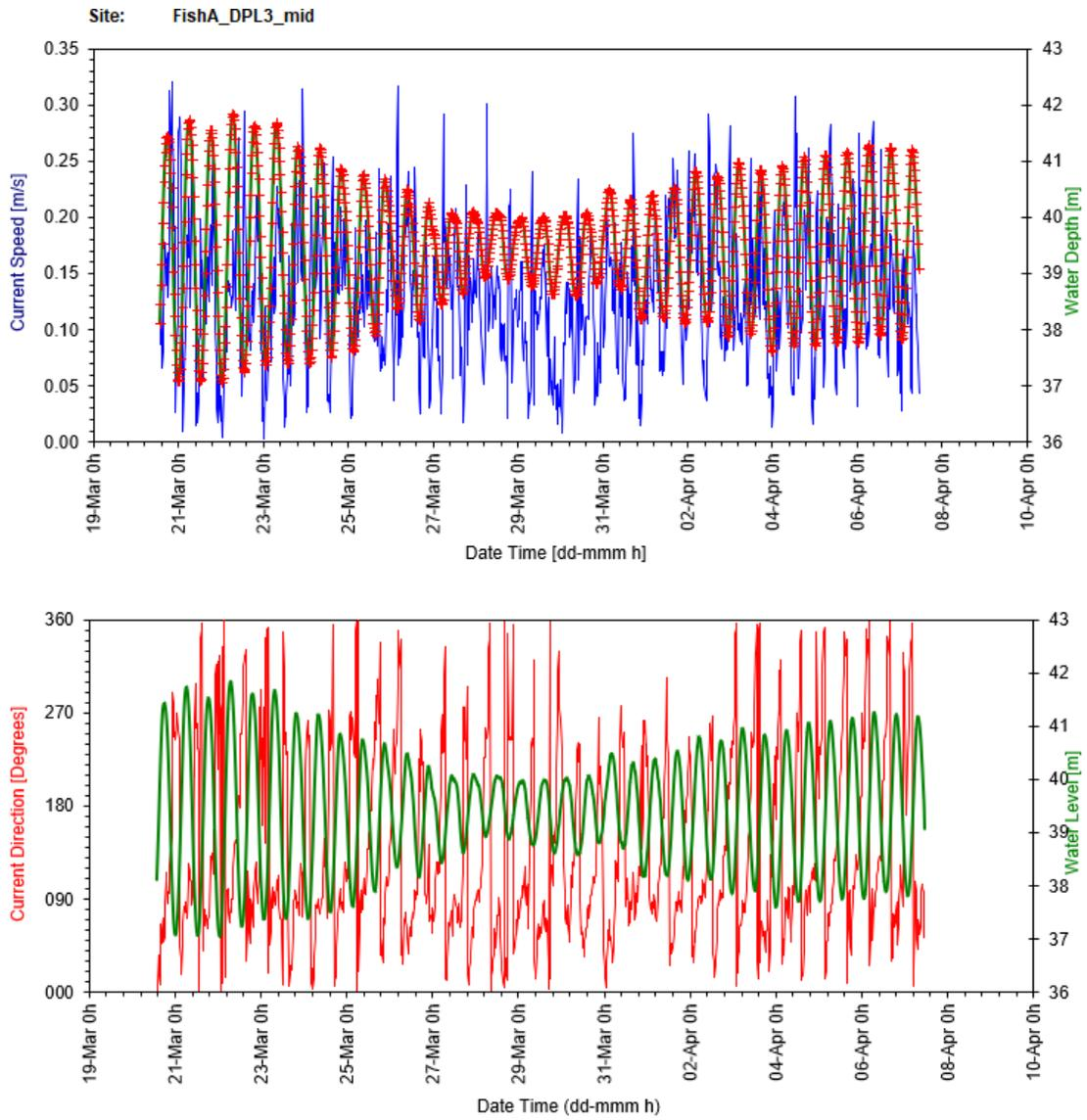
Figure 6: Cage bottom time series plots for current speed and direction against water level
