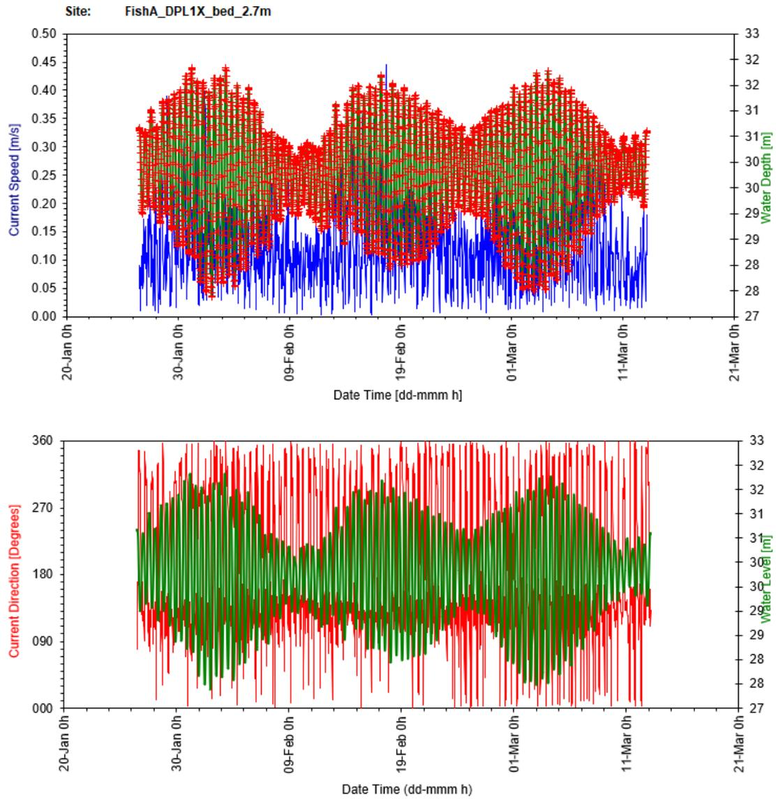
Figure 23: Near-bed time series plots for current speed and direction against water level
