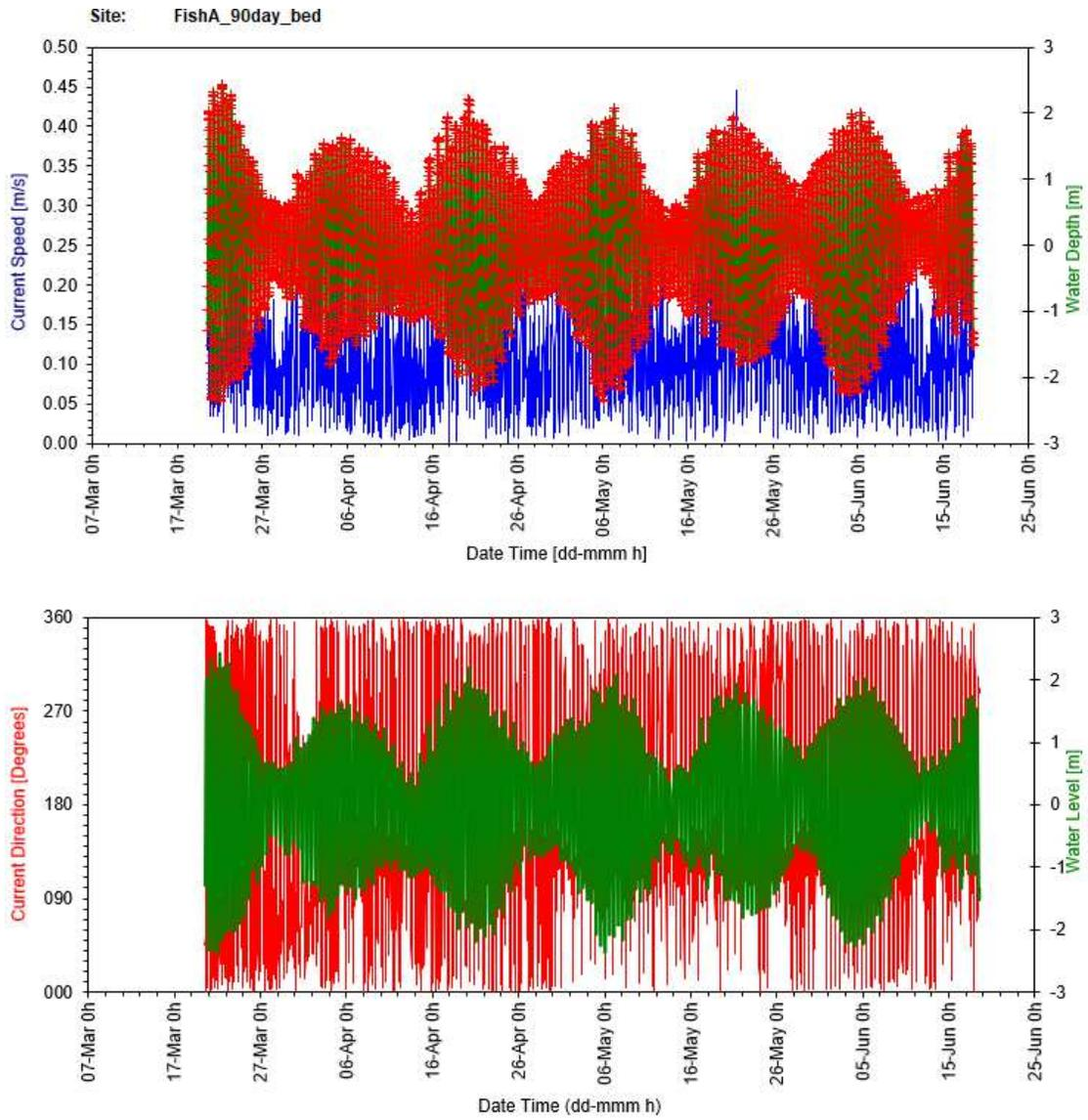
Figure 32: Bed time series plots for current speed and direction against water level
