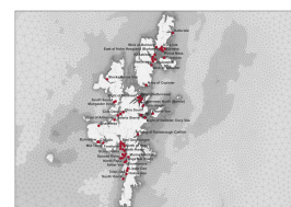
Area of interest and computational mesh of East of Shetland hydrodynamic model
