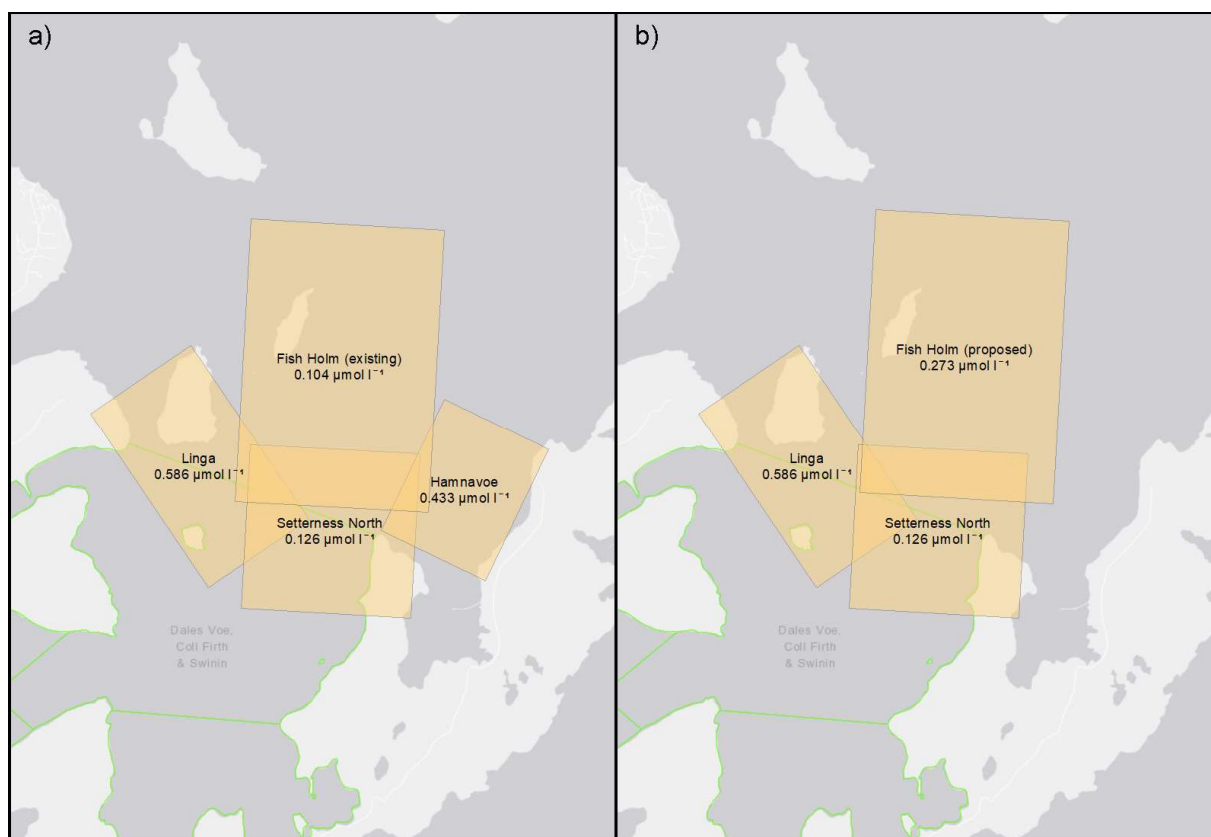
Figure 2 Indicative plume extents and maximum ECE for a) the existing scenario, and b) following expansion at Fish Holm, including relinquishment of the Hamnavoe CAR licence. The Swinister Voe categorised area is demarked with the green line.
