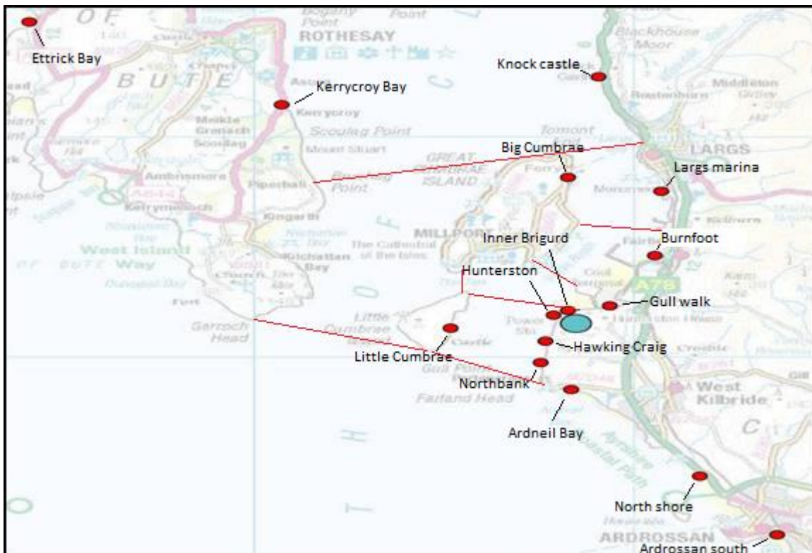
Figure 62 – Hunterston district sampling locations for sediment and seaweed (red circles), shown with GoldSim model compartments (red lines). Adapted from reference [41].
