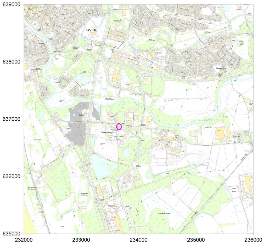
Figure 15 98.08 th Percentile 24-Hourly Average Process Contribution Due to Short-Term Releases of PM 10 ( \mu\text{g m}^{-3} ); 2016 Meteorological Conditions. Magenta Isopleth Denotes the Point of Insignificance (10 % of the AQS)
