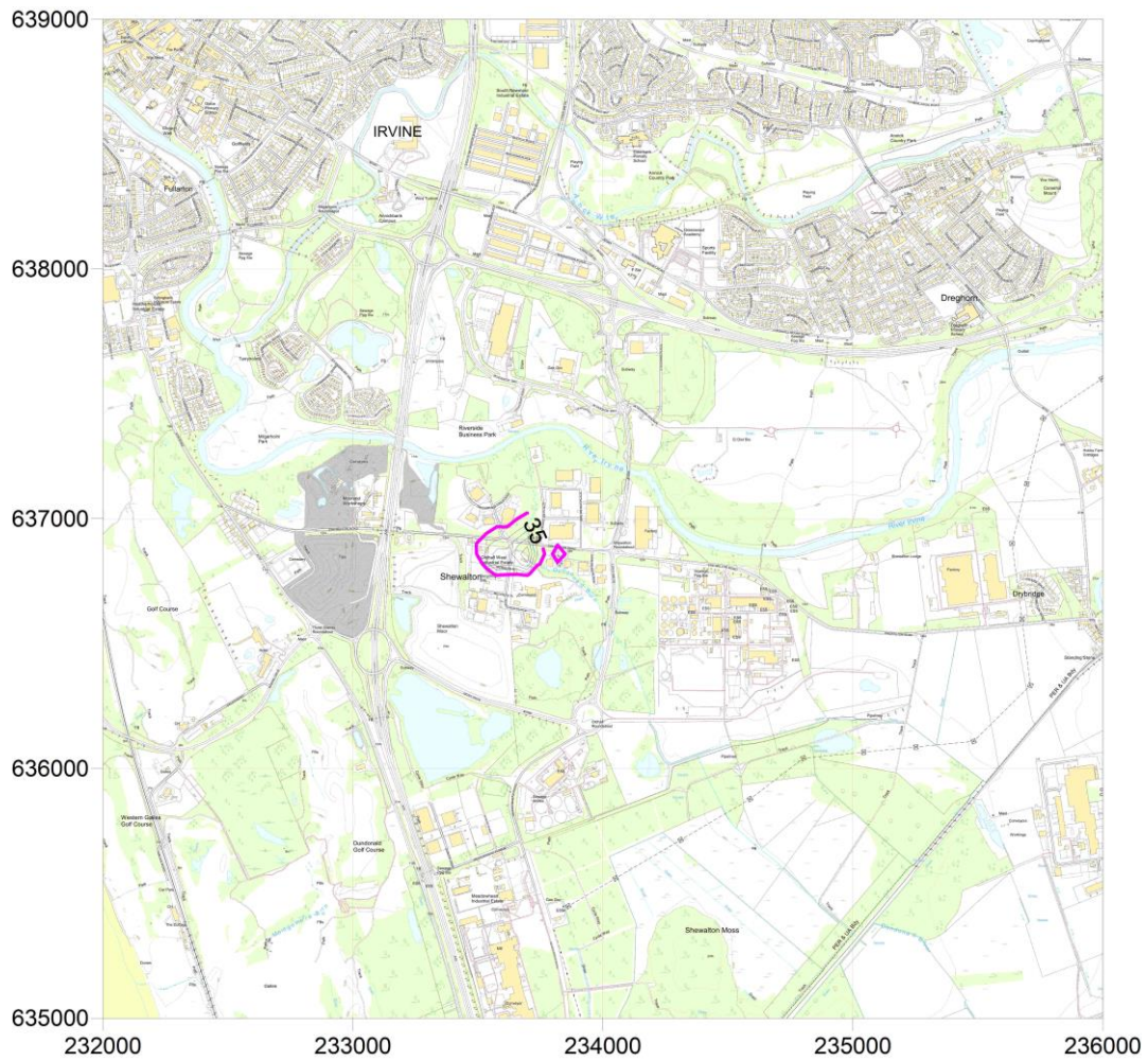
Figure 14 99.73 rd Percentile Hourly Average Process Contribution Due to Short-Term Releases of SO 2 (µg m -3 ); 2016 Meteorological Conditions. Magenta Isoleth Denotes the Point of Insignificance (10 % of the AQS)
