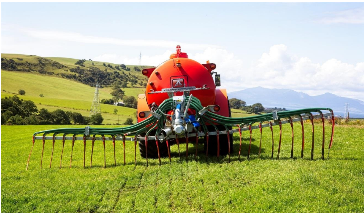
Precision application: trailing hose application of slurry at Low Ballees Farm, West Kilbride
